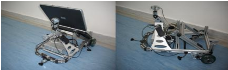
Fig. 1. Chassis Evolution robotics platform ER1.
