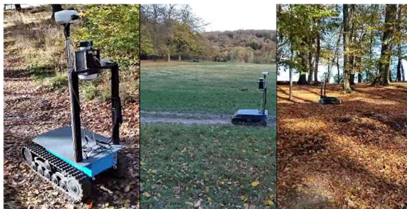
Fig. 2 RTV Crawler mobile platform with sensoric setup in different environments during recording of our dataset Source: author.
