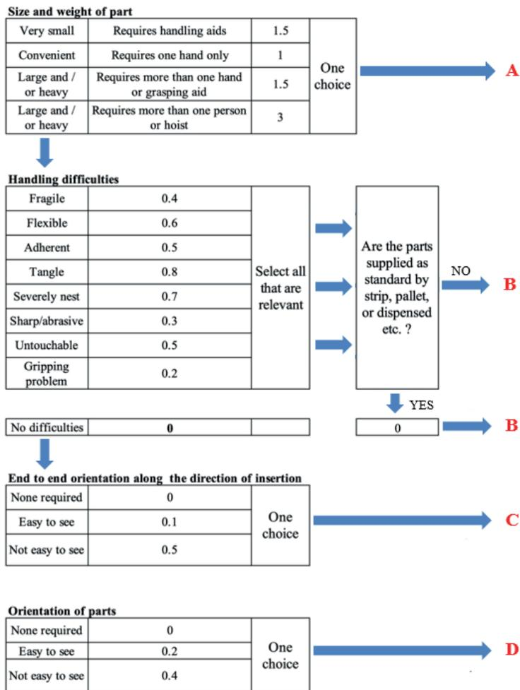
Figure 8 Manoeuvring analysis scoring diagram in LUCAS DFA [18-19]
