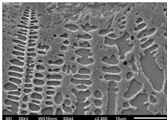
**Figure 7** Image showing the alloyed zone (sample 2 after alloying 40 A)
