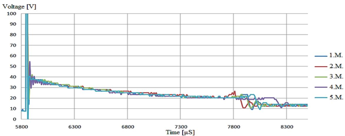
**Figure 14** The course of voltage during the arc burning by applying gasoline
