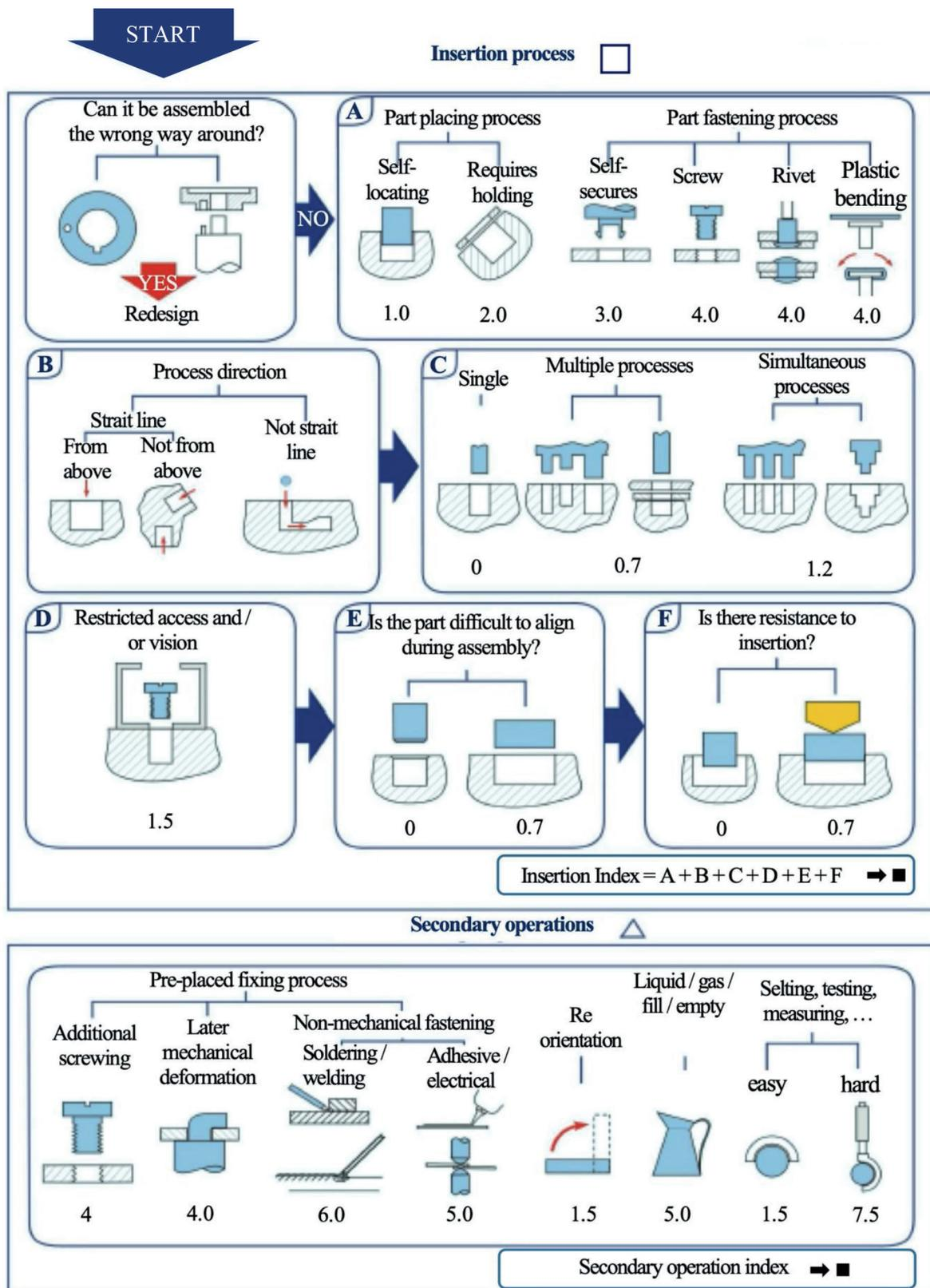
Figure 9 Assembly analysis scoring diagram in LUCAS DFA [18]
