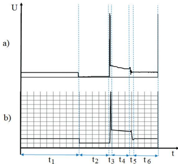
Figure 7 Voltage waveform on the primary part of the ignition module: a - real, b - simulated
