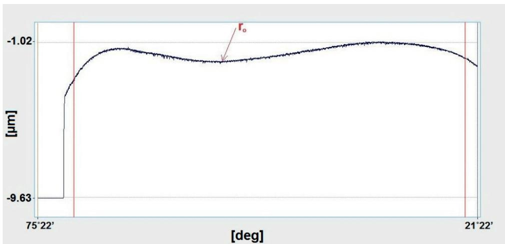
Figure 5 Outer race profile measured using the STPP system
