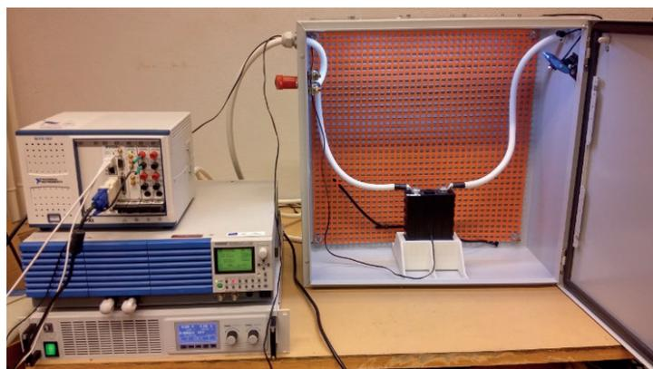
**Figure 2** Experimental test-stand for the traction batteries recovery
