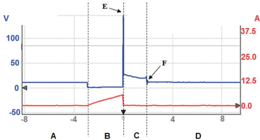
**Figure 6** Current and voltage waveforms on the primary side of the ignition module:
