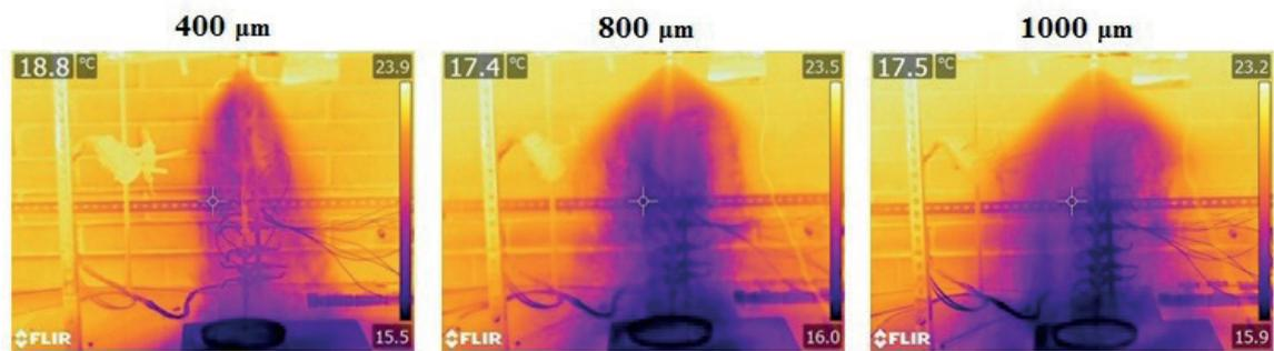
Figure 4 The spraying characteristics of the tested nozzles (thermogram)
