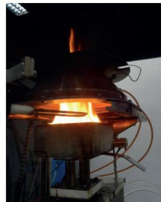
**Figure 2** MARHE determination using a cone calorimeter according to ISO 5660-1
