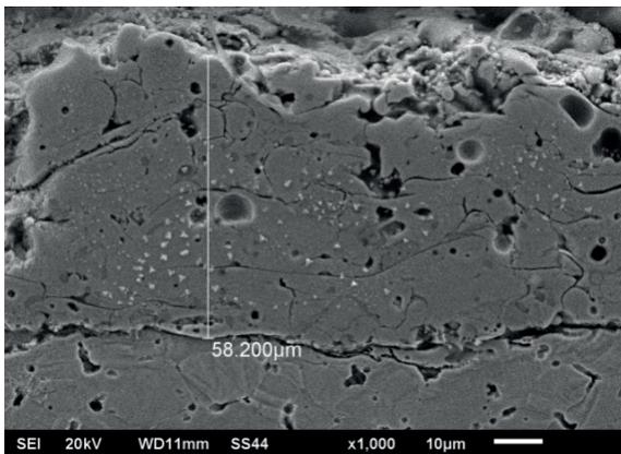
**Figure 4** SEM image of the coating after APS
