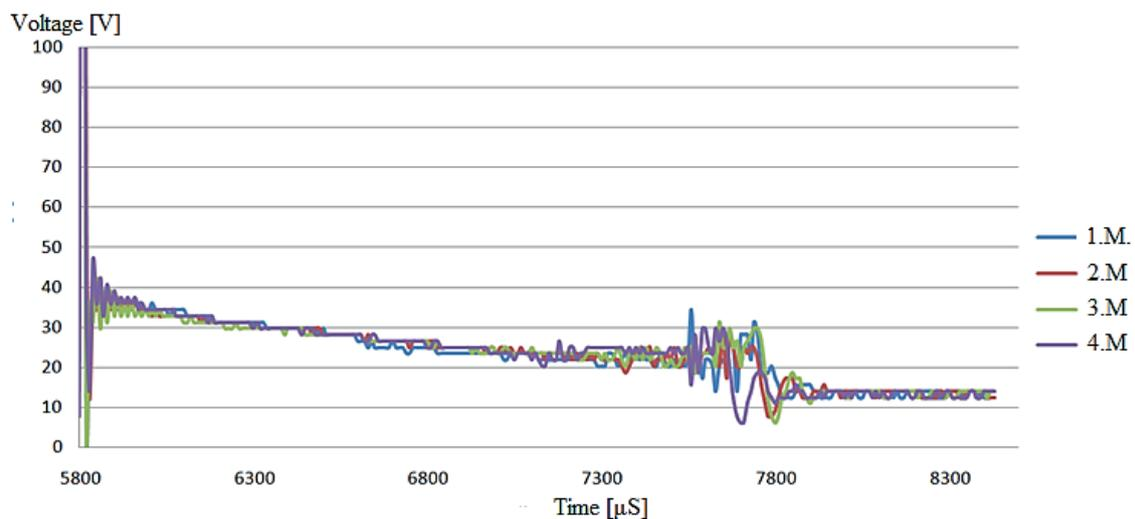
**Figure 15** The course of voltage during the arc burning by applying oil
