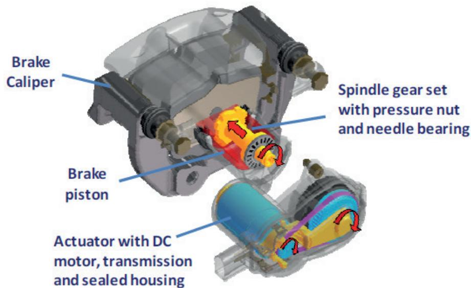
*Figure 4 Mechatronic EPB actuator and caliper assembly [1]*
