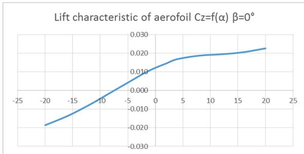
**Figure 6** Aerodynamic coefficients power of lift obtained during the measurements for the slip angle  $\beta = 0^\circ$
