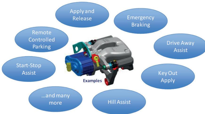
Figure 2 Functionalities of the Electric Parking Brake
