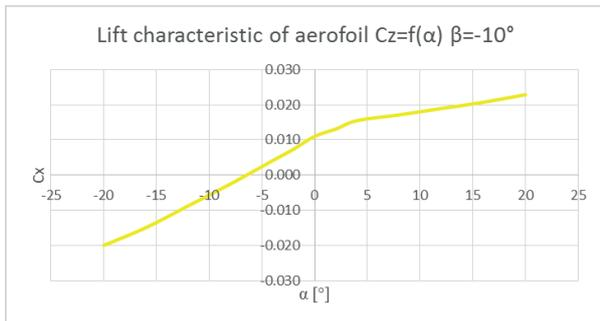
**Figure 7** Aerodynamic coefficients power of lift obtained during the measurements for the slip angle  $\beta = -10^\circ$
