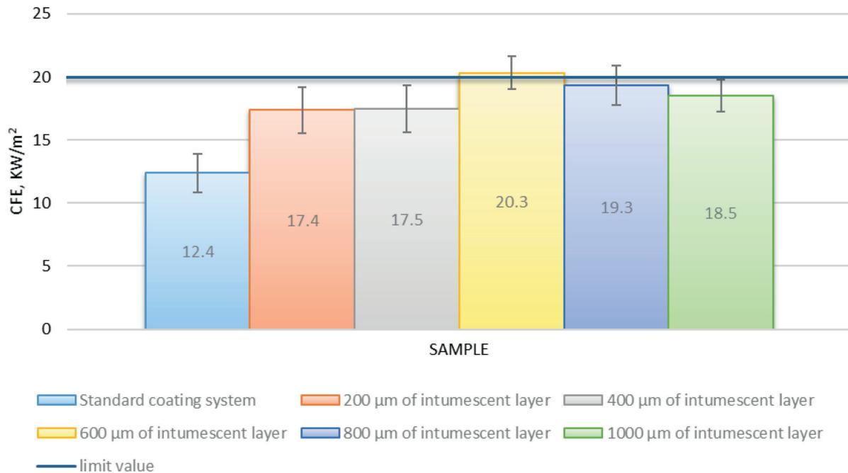
**Figure 6** Results of the critical heat flux of the coating system after applying a fire protection layer of varying thickness
