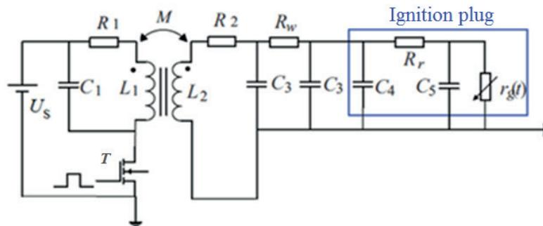
Figure 3 The replacement model of the ignition assembly
