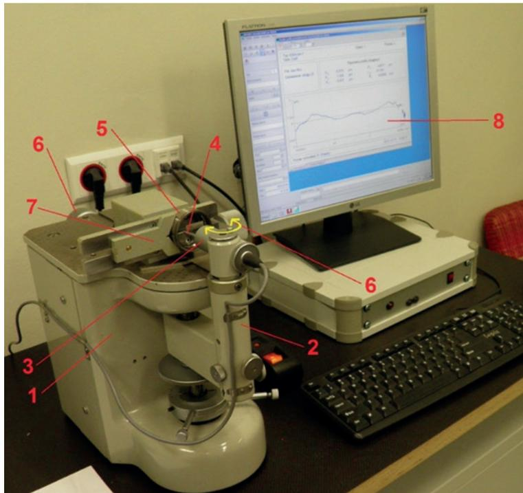
**Figure 3** STPP measuring system for analysis of the geometry of bearing raceways:
