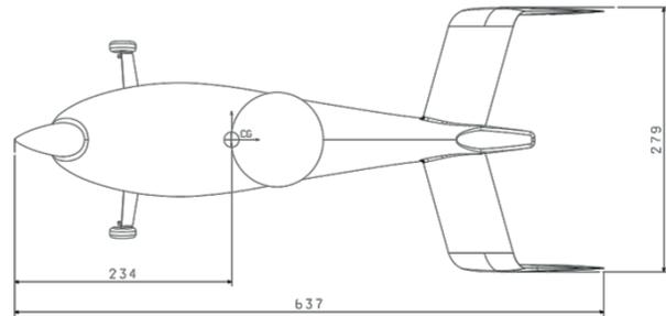
**Figure 3** Upper view of the gyroplane
