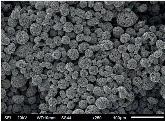
**Figure 2** Grains of the  $Cr_3C_2$ -NiCr powder
