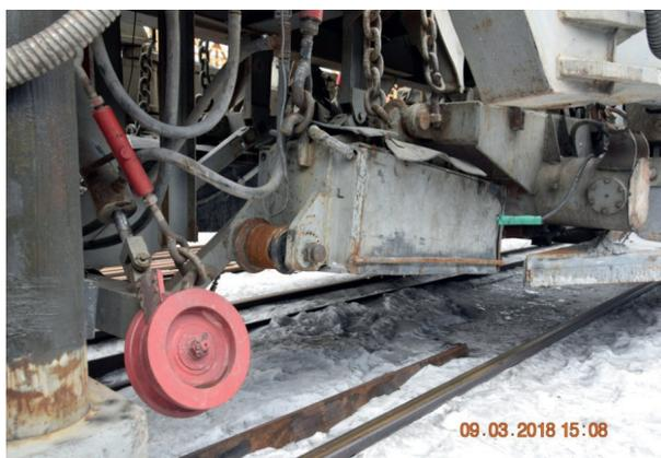
**Figure 3** Electromagnetic grippers of the VPO-3-3000 machine
