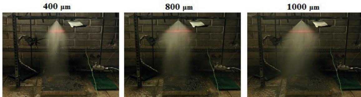
Figure 3 The spraying characteristics of the tested nozzles
