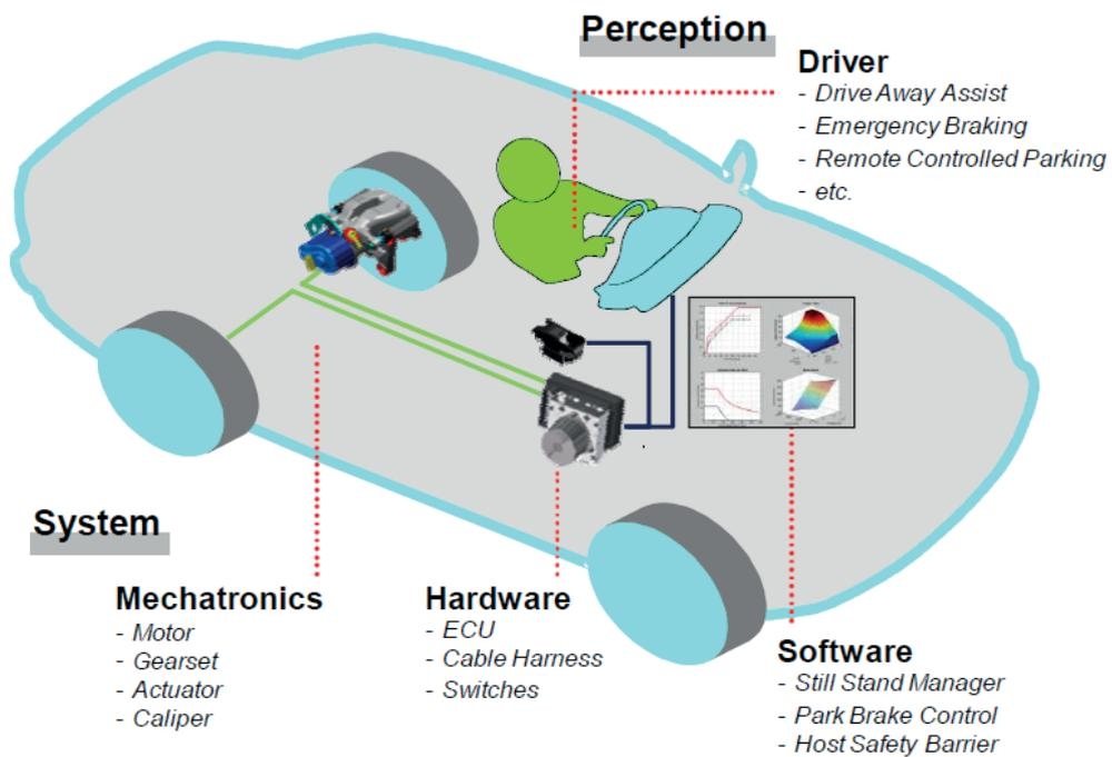
Figure 3 Electric Parking Brake System (EPB)
