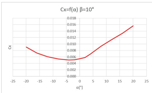
**Figure 8** Aerodynamic coefficients power of drag obtained during the measurements for the slip angle  $\beta = 10^\circ$
