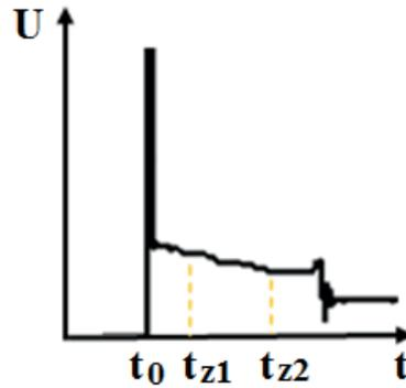
Figure 10 Arc burning interval with two sampling points
