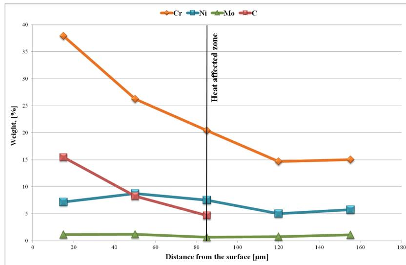
**Figure 8** Linear chemical composition analysis for sample 2 after alloying at current intensity 30 A
