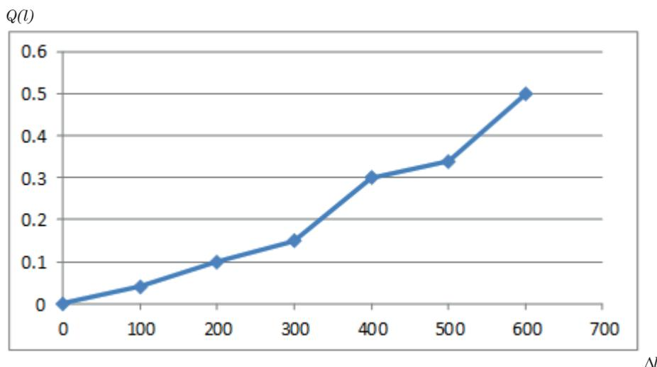
**Figure 2** Probability of the electromagnetic grippers failure  $Q(l)$  in terms of the operating time  $\Delta l$ , km
