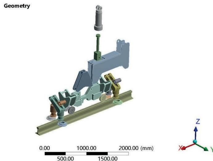
**Figure 5** Three-dimensional assembly model of the LLD (lifting-leveling device) design
