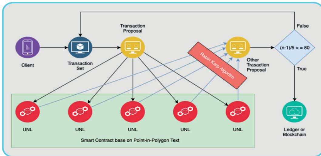
Figure 5 Design of the RPCA in This Research
