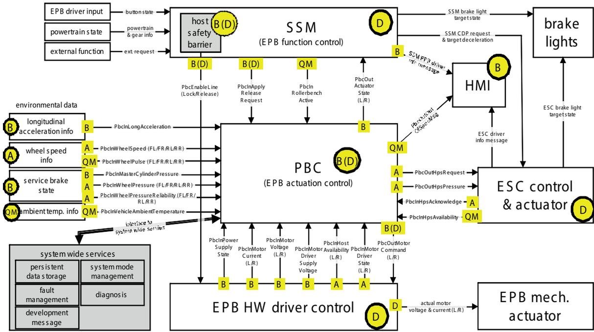
Figure 8 Overview of EPB functional architecture with relevant ASIL levels (maximum overall hazards, hazard 1a according to ASIL B(D) and ASIL B(D) decomposed) signals
