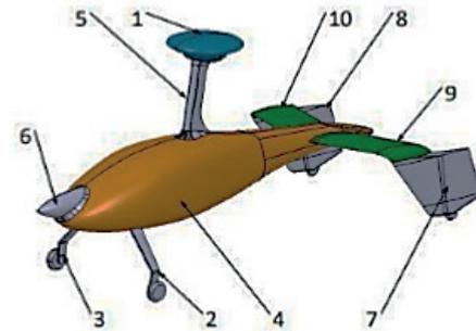
**Figure 4** Specification of a gyroplane: 1 - head, 2 - left shank, 3 - right shank, 4 - hull, 5 - pole, 6 - nose, 7 - left vertical stabilizer, 8 - right vertical stabilizer, 9 - left horizontal stabilizer, 10 - right horizontal stabilizer
