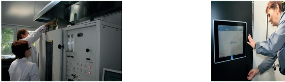
**Figure 3** Determination of smoke properties using a smoke chamber according to EN ISO 5659-2 and a toxicity index when connected to the FTIR analyzer chamber (on the right) according to EN 45545-2 Annex C
