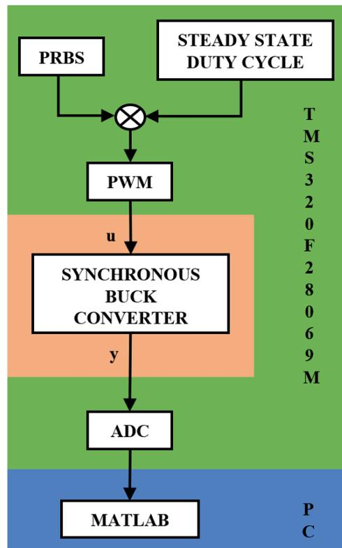
**Figure 1** Block schematics of the experiment, where  $u$  is input and  $y$  is output of the system
