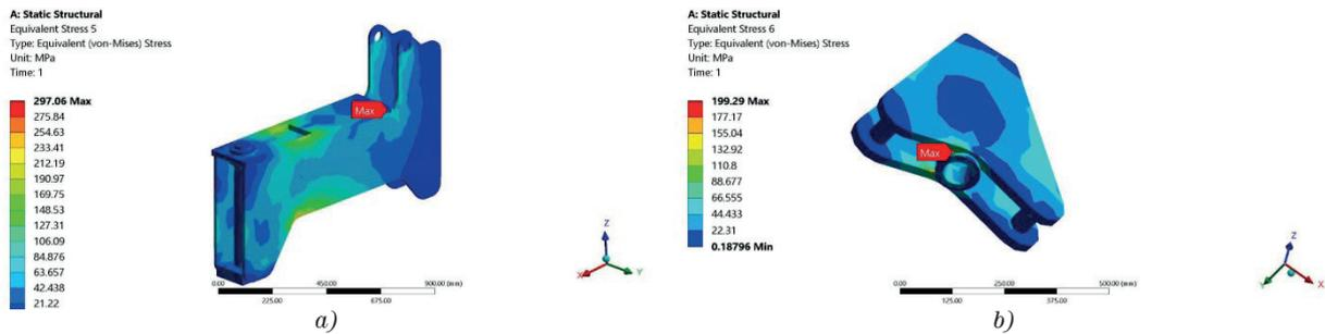
Figure 13 Stresses according to Mises: a) front right gripper; b) front left gripper
