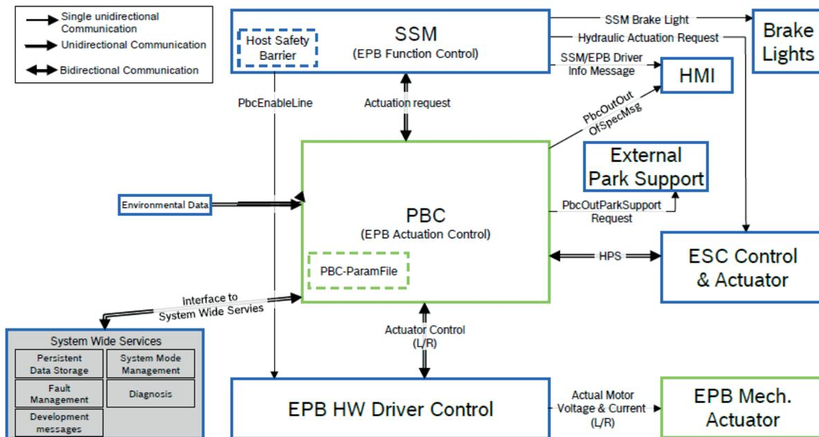
Figure 7 Overview of the functional architecture of the integrated EPB system including interfaces [6]
