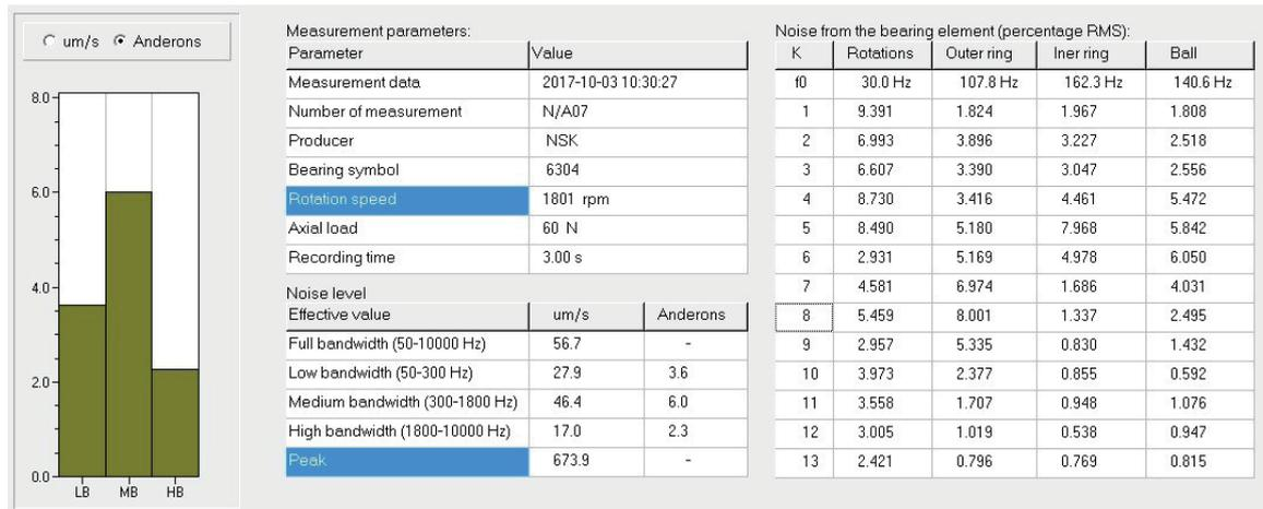
Figure 2 Measurement report obtained from Anderonmeter software
