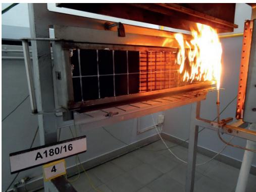
**Figure 1** Determination of Critical Flux at Extinguishment- CFE according to ISO 5658-2
