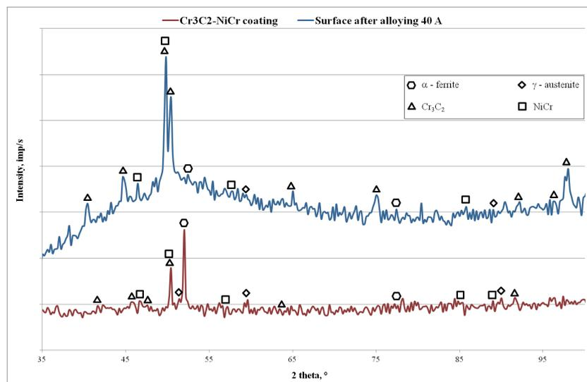
**Figure 9** Diffractograms of sample 3 with  $Cr_3C_2$ -NiCr coating after alloying (40 A)
