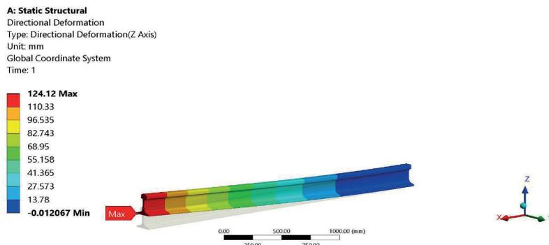
Figure 10 Vertical strain of the R75 rail
