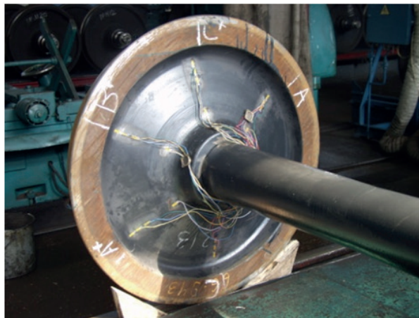
Figure 8 Measuring scheme on the experimental wheel pair
