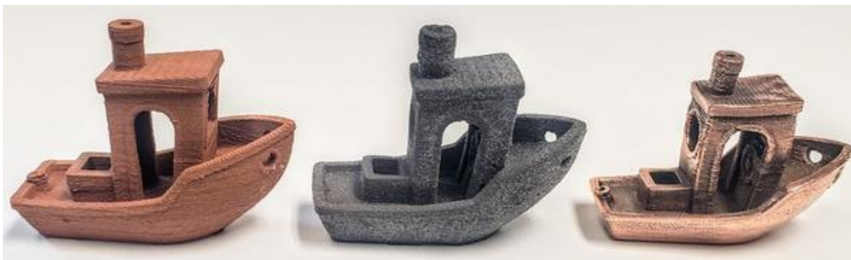
Fig. 1 3D model of a ship made of unfired copper, after descaling and sintering [source: The Virtual Foundry]
