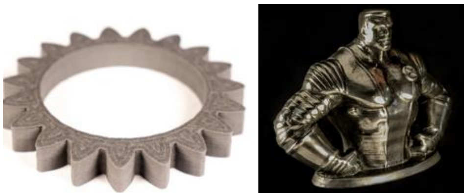
Fig. 2 Gear made of 316L stainless steel without sintering and Model manufactured with Filamet™ 316L stainless steel and sintered [source: The Virtual Foundry]
