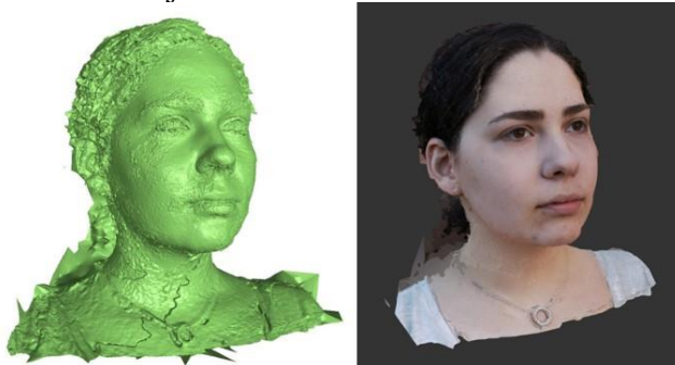
Fig. 3 Display of STL model in GOM (left) and model in RealityCapture software (right).
