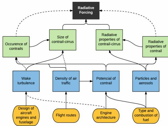
Fig. 1 Structure of elements, which influence contrail formation and subsequent radiative forcing
