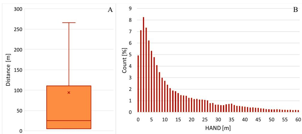
Fig. 2. A – Distance of segregated MRCs (calculated from the nearest point of the polygon) to the nearest watercourse (ZB GIS). Whiskers length is:  $1.5 \times (Q_{75} - Q_{25})$ , B – Distribution of heights above the nearest drainage (HAND) computed over all pixels covering the MRCs
