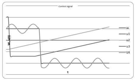
w - learning objectives, u1, ..u4 - control signals Fig.2. Change of control signal
