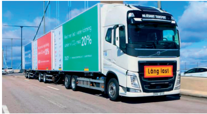
Figure 1 Road train with two trailers [9]
