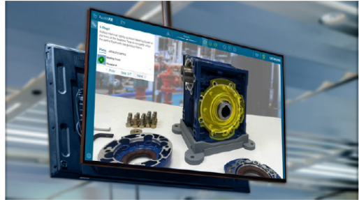
Fig. 1. Demonstration of Assist AR when disassembling the gearbox [5]
