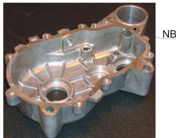
Figure 15. Verified machine part—gearbox cover with marked zero point (ZP).
