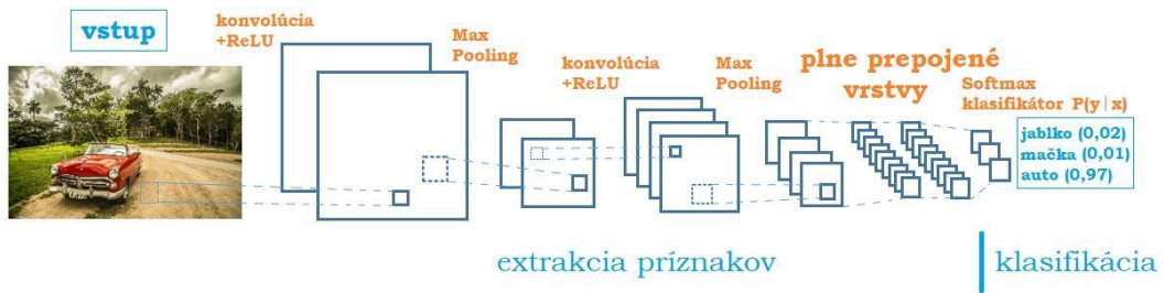
Fig.5. Simplified CNN operation procedure [8].
