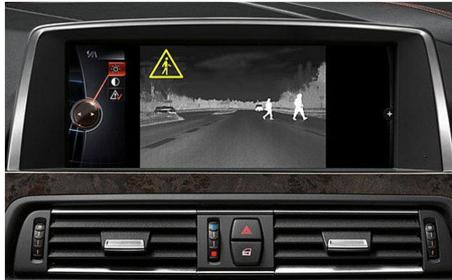
Fig.1. Detection of people on the road using an infrared camera [4].
