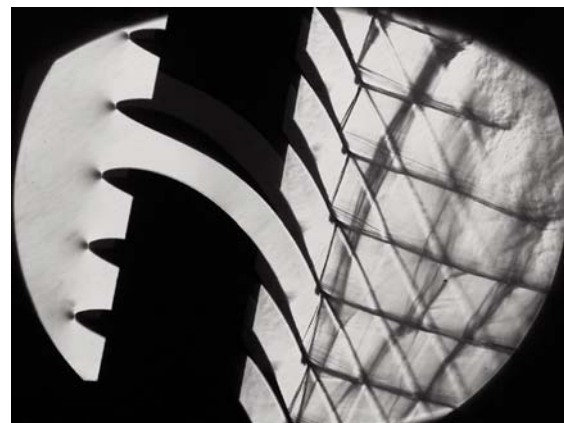
Fig. 3 The schlieren picture of the flow field in a profile cascade, i = 0^\circ , M_{2is} = 1.402 . Additional shock waves appear in the exit flow field which is therefore disturbed and aperiodic
