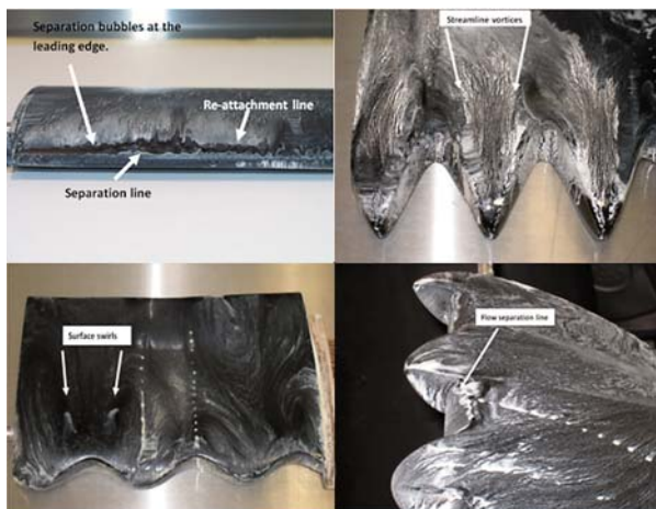
Fig. 6 Flow visualization of the models at 18 degrees angle of attack and Re = 3.3 \times 10^5 . Baseline (top left) Configuration 1 (top right) Configuration 2 (bottom left) and Configuration 3 (bottom right)
