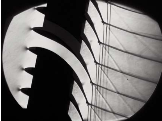
Fig. 4 The schlieren picture of the flow field in a profile cascade, \iota = 0^\circ , M_{2is} = 1.828 . No additional shock waves visible, perfect flow field periodicity in exit part of interblade channels
