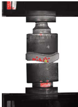
Fig. 3 Tearing of the test specimen
