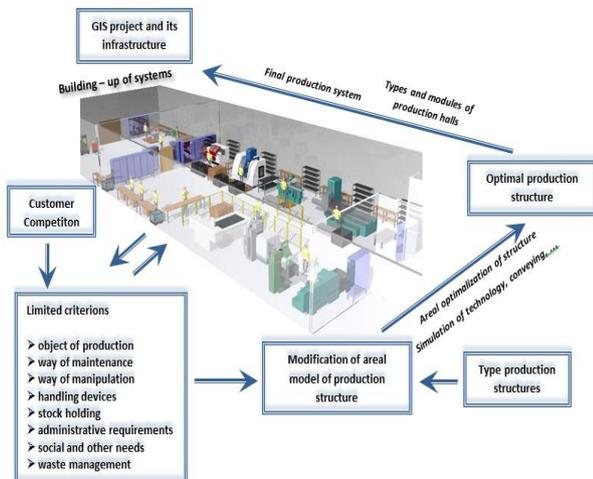
Figure 1 Design procedure characteristics of new production structure
