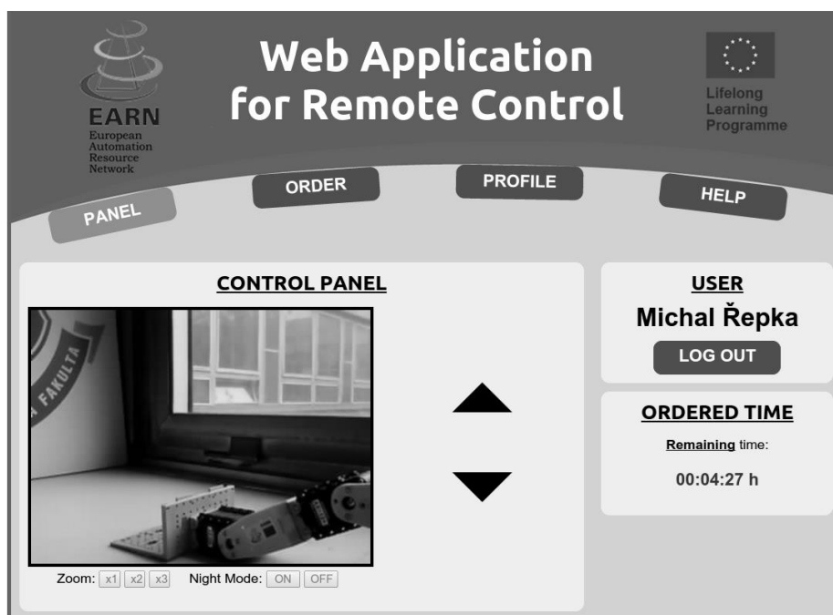
Figure 3 Web application for the remote control of the Bioloid robot (Černín, 2014).
