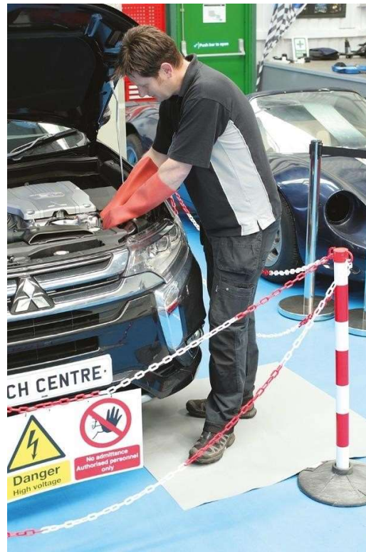
Fig. 3.15 Maintenance work on EV with usage of protective gloves, source: archive e-Tech Systems Engineering s.r.o
