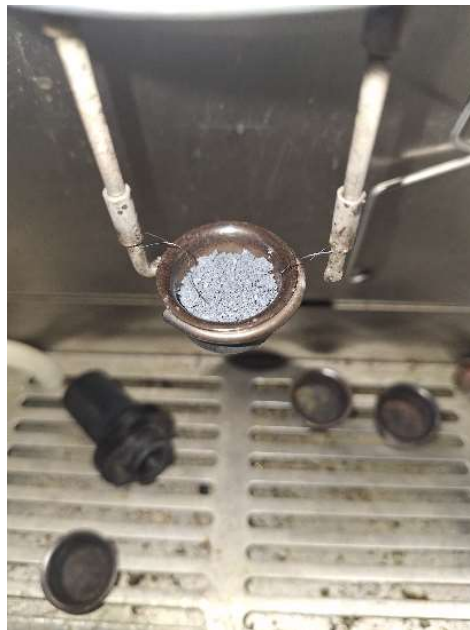
Fig. 8.10 Measuring vessel with weighed waste sludge sample with embedded ignition wire
