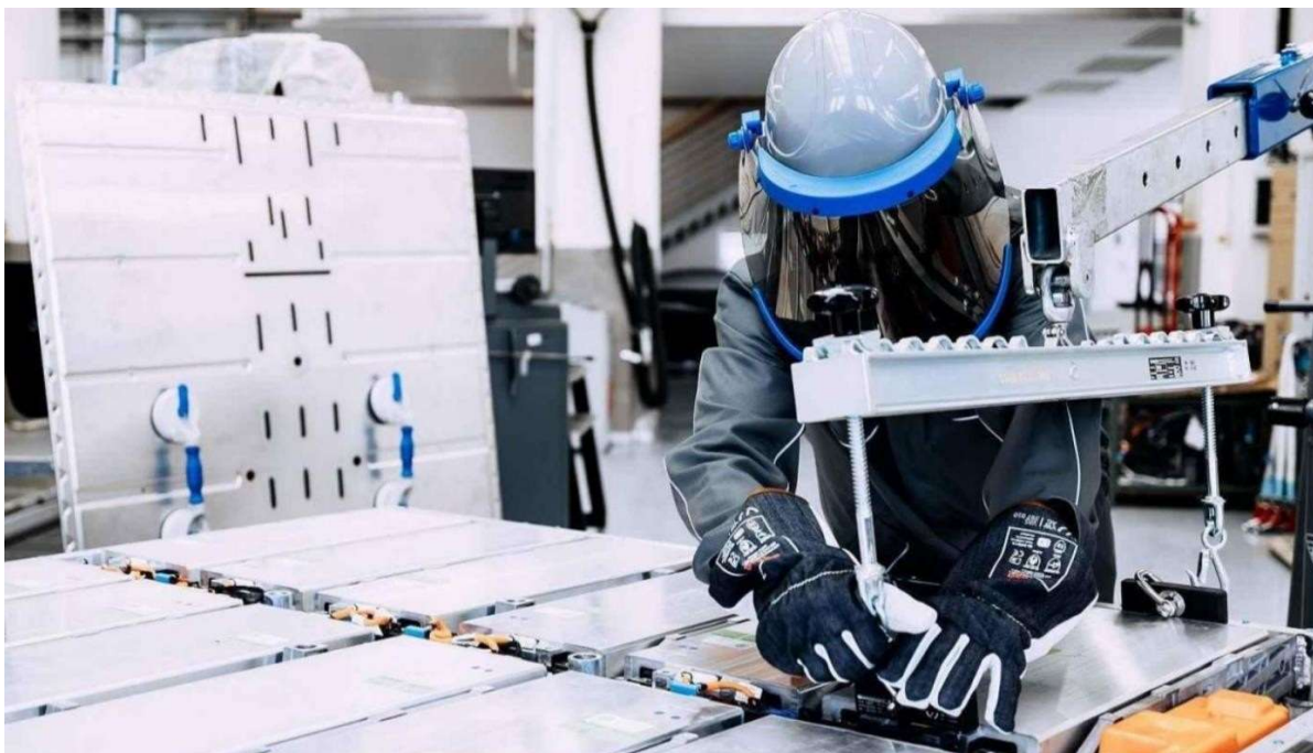
Fig. 3.16 Maintenance work on EV with usage of protective gloves and eye protection shield [3].
