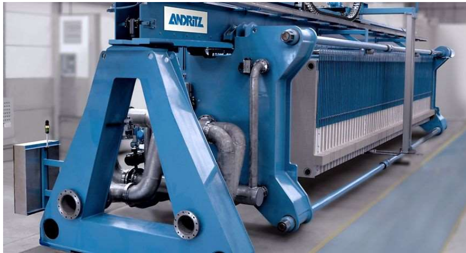
Fig. 8.6 Chamber sludge press with upper suspension – beam (Andritz)
