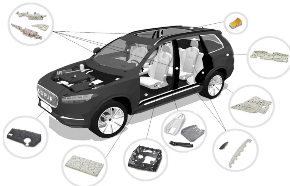
Fig. 4.18 Acoustic infill in vehicle interiors and infill for car seats.
