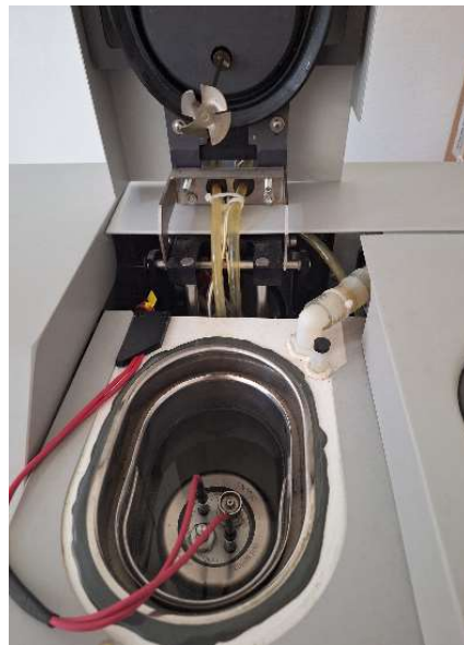
Fig. 8.12 Sample ready for calorific value measurement in the calorimeter
