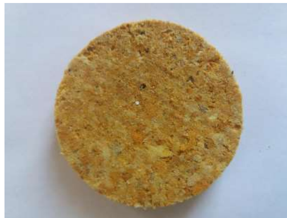
Fig. 4.21 Resulting moulded element at optimum process conditions (200 °C; 5.7 kPa; 12 min endurance).
