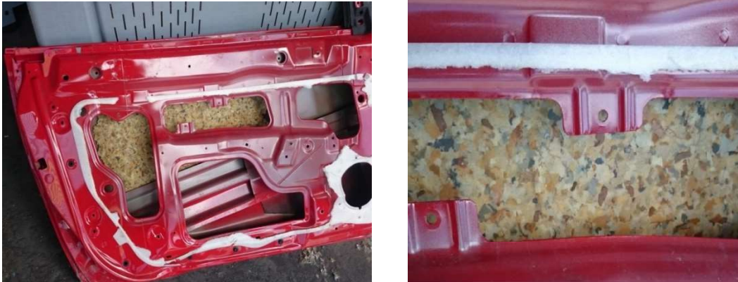
Fig. 4.10 Insulation for vibration damping in cars.
