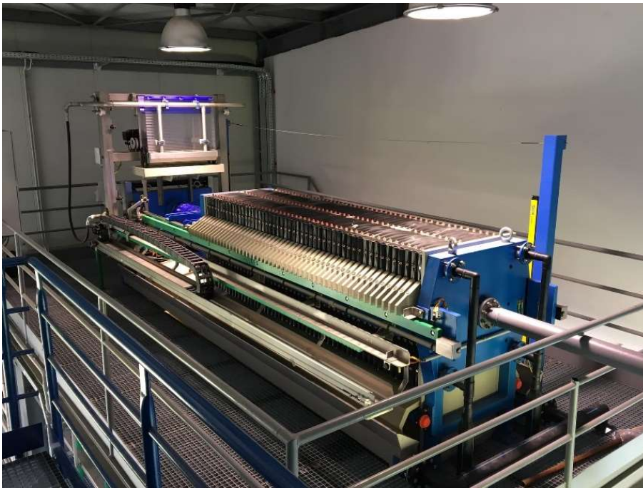
Fig. 8.5 Chamber sludge press with side connecting rods (Envites)
