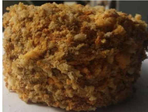
Fig. 4.20 Non-compliant moulding under inappropriate process conditions (150 °C; 2.0 MPa; 12 min endurance).
