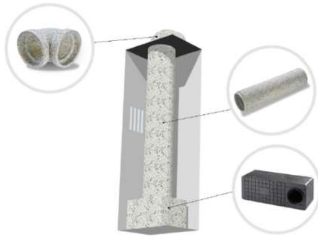
Fig. 4.17 Acoustic infill in exhaust and ventilation systems, thermal insulation of duct systems.
