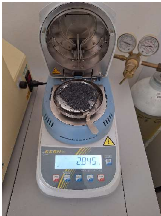
Fig. 8.7 Sample ready for drying in the KERN drying scale
