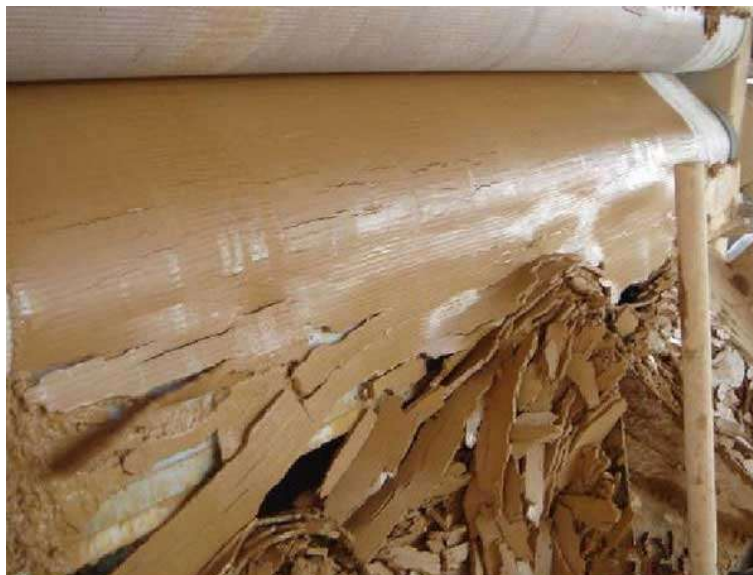
Fig. 8.4 Output of the band sludge press ( www.filterpressmachine.com )
