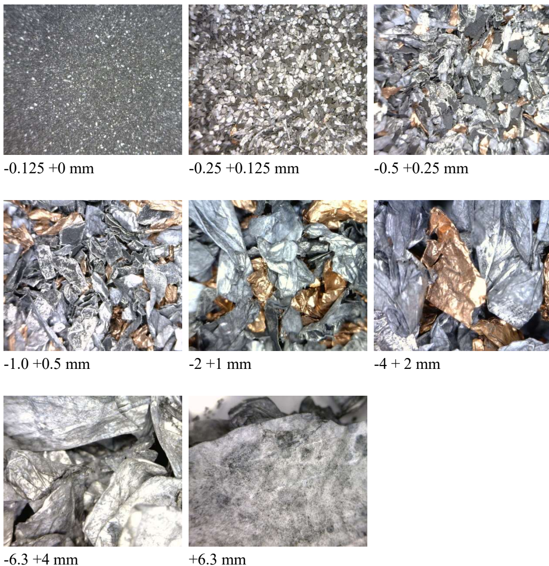
Fig. 5.5 Detailed view of grain size fractions at 50x magnification
