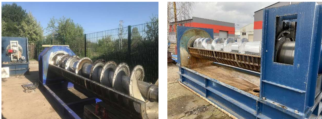
Fig. 8.2 Threaded sludge press (IEA Press)
