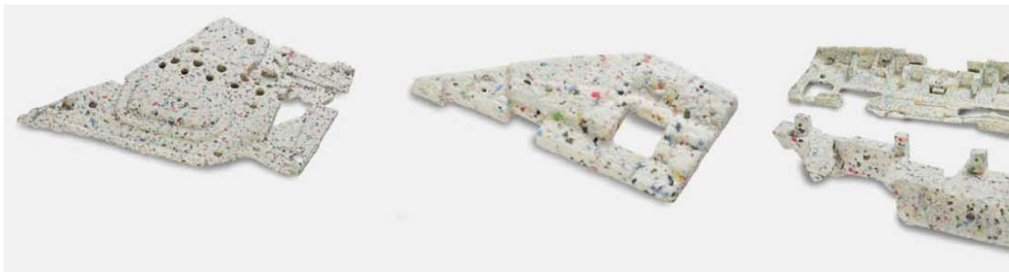
Fig. 4.11 Complex shaped parts from recycled PUR foam.
