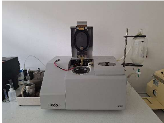
Fig. 8.9 LECO AC500 calorimetric instrument for measuring calorific value of fuels
