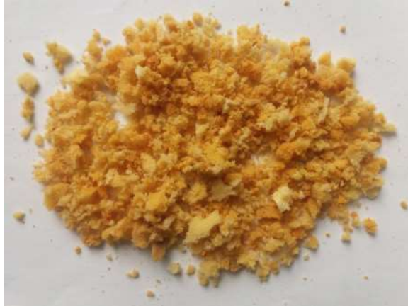
Fig. 4.19 Size fraction of the crushed PUR foam (2.0 – 15.0 mm).
