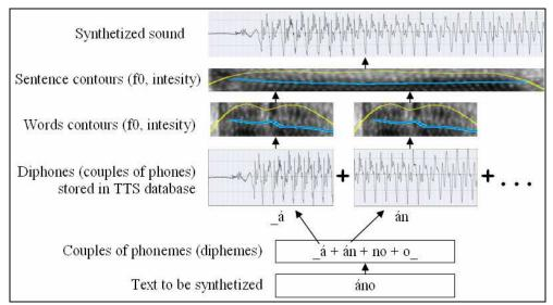
Fig. 1. Concatenative method of speech synthesis in the TTS-KIS system, based on speech synthesis unit "diphone".
