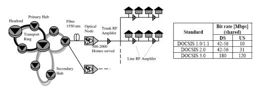
Fig. 4. Architecture HFC network
