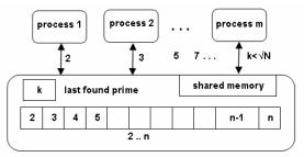
Fig. 1. Schema of parallel algorithm on shared memory
