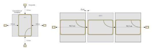
Fig. 4. Maximum transponder identification range of a single and three antenna areas
