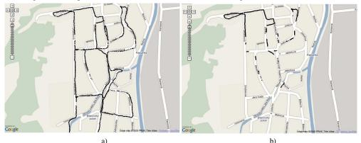
Fig. 3. a) Radio map database with all spots; b) Radio map database filtered for BS with CID=4F81, BSIC=29 and BCCH=15.
