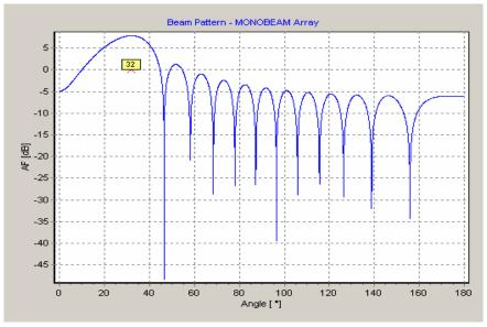
Fig. 1. Monobeam array beam pattern.
