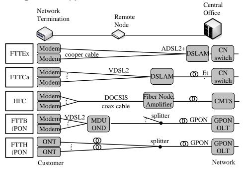
Fig. 1. Access Network, technologies xDSL, HFC, FTTx.
