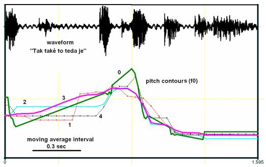
**Fig. 7.** Choosing the best method of smoothing. Contours of the sentence "Tak, také to teda je". Stress is on the word "také" ( – contour from Praat, 1 – Moving average (given interval length), 2 – Moving average (given number of points), 3 – Weighted moving average (given number of points), 4 – Exponential smoothing).
