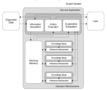
Fig. 4. Extended architecture using common working memory.
