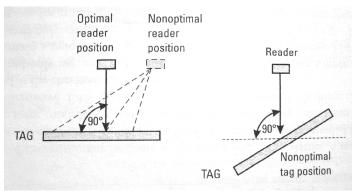
Fig 1. Optimal and nonoptimal tag and reader position [1]
