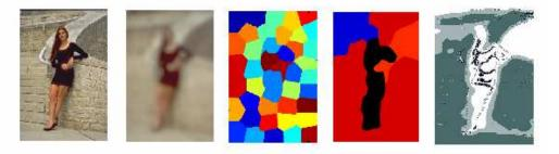
(a) (b) (c) (d) (e) **Fig. 1.** Progress of perceptual image segmentation algorithm: (a) original image; (b) result of perceptual tower; (c) result of k-means segments; (d) result of merged segments (e) result of final segments after segmentation
