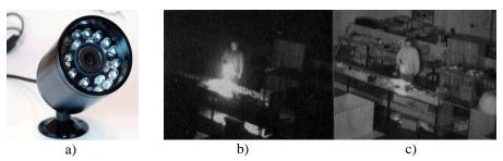
Fig. 1 a) IR illuminated camera, b) Scene without IR, c) Scene with IR
