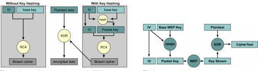
Fig. 1. Temporal key integrity protocol (TKIP).
