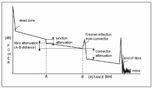
Fig. 5. Reflectogram of the examined length.
