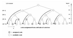
Fig. 2. LCA assignment scheme.
