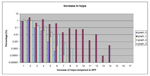
Figure 1: Increase in the number of hops compared to the shortest path when using FIFR-N algorithm (percentages on logarithmic scale)
