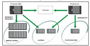
Fig. 2. The reference between Profinet CBA and Profinet IO
