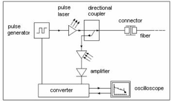
Fig. 3. Diagram of reflectometer.
