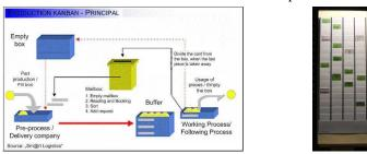
Fig. 1. Transportation Kanban Process[1] and "Sm@rt Logistics" Singlearea-eKanban Board
