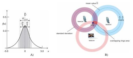
**Fig. 1.** The figure A) the gauss curve expressed distribution of distance estimation between node an beacon and the possible mistake of measurement. The figure B) the field (area) of possible occurrence, where the node could be located. It is limited by beacon realization of beacon rings (overlapping).
