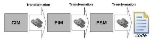
Fig 1. Concept of Model Driven Architecture. Development of an information system on various levels of abstraction.
