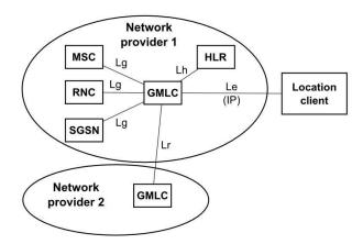
Fig. 1. Architecture of location system.
