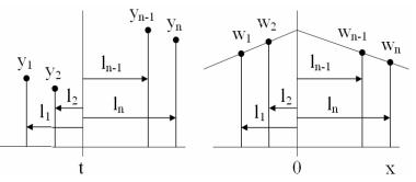
Fig. 5. Computing weights in Method 3: Weighted moving average (given number of points).
