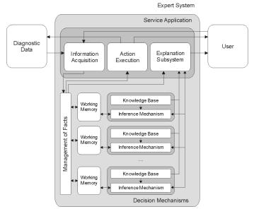
Fig. 5. Extended architecture using separated working memories.
