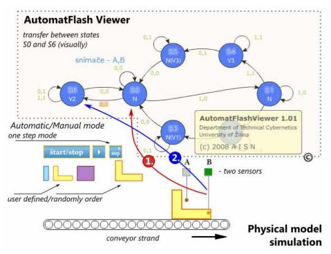
Fig. 2. Interactive flash application for three different products recognition based on AutomatFlash Viewer.
