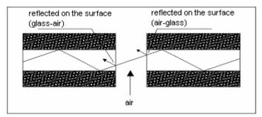
Fig. 2. Phenomenon of Fresnel's reflection.
