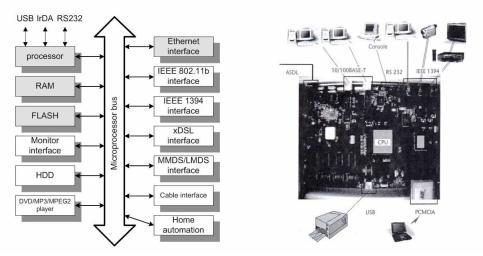
Fig. 4. Compact hardware architecture.
