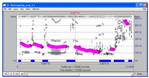
Fig. 3. Melody contour computed by "To Pitch (ac) "method of program Praat (default settings: analyzed frequency range 75 Hz - 600 Hz).
