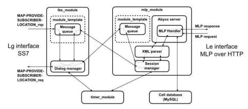
Fig 2. Scheme of lbs\_module and mlp\_module.
