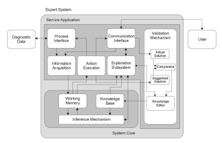
Fig. 3. Architecture of knowledge system extended by validation mechanism.
