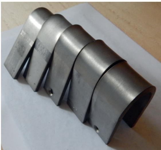
Figure 1 Samples after bending
