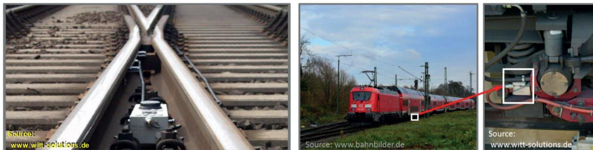
Figure 1 The inertial measurement systems (left - ESAH-M, right - ESAH-F)
