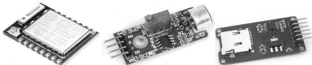
Fig. 2. Wi-Fi module ESP8266-07, microphone module, SPI - reader module for micro SD card.
