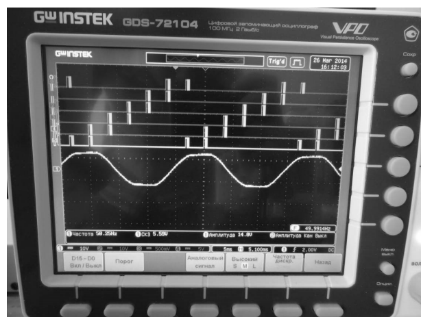
Fig. 7. Oscillogram of phase A of the supply network and 6 channels at the output of the control system with a pulse width of 650 mks.
