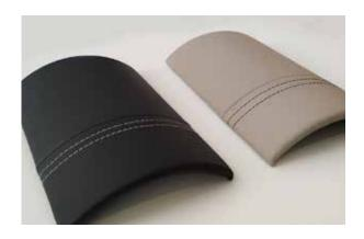
The Nanocleanleather project set out to develop leather with anti-soiling properties (dirt-repellence and easy cleaning) and self-cleaning (photocatalytic degradation of contaminants on the surface of the leather) for the automotive sector (specifically seat covers, steering wheels, dashboards and door panels) using nanostructured additives.
