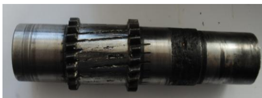
Figure 2. The pinion damage.
