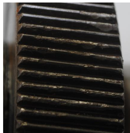
Figure 4. Damage to the teeth of gear wheel.
