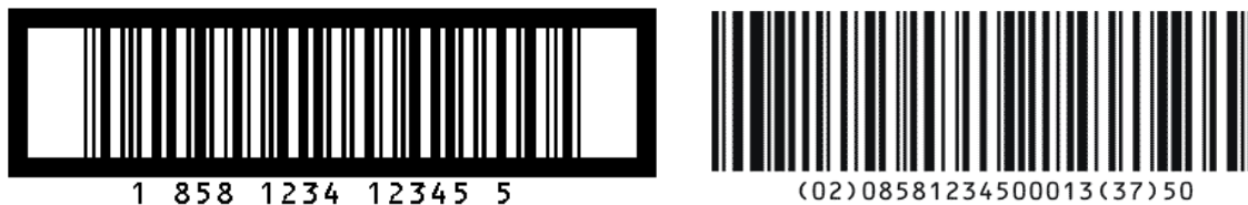
Fig. 1. Bar code ITF-14 (left) and GS1-128 (right).
