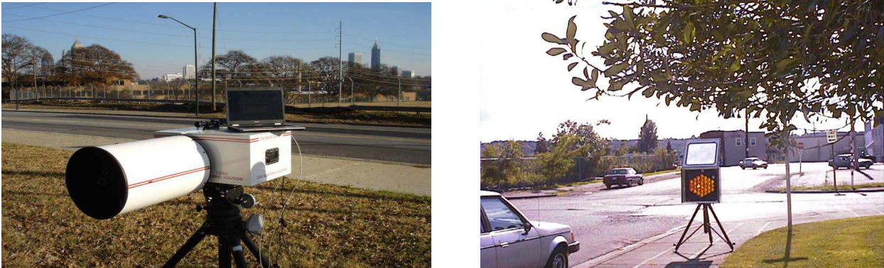
Fig. 3. Open-Path AirSentry FTIR system [4]
