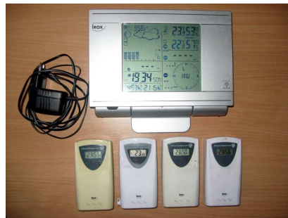
Fig. 2 The Meteo station Irox PRO-X USB with sensors
