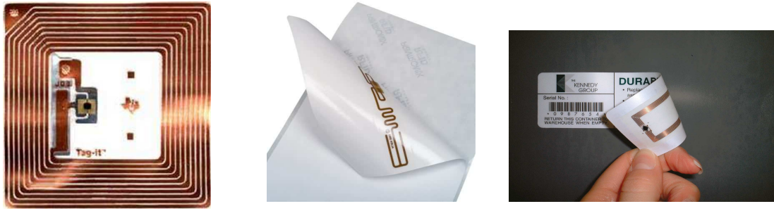
Fig. 2. RFID chip and RFID chip as a self adhesive label.
