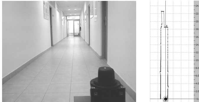
Fig.1. Space of the hallway scanned by sensor and graphic representation of measured values.
