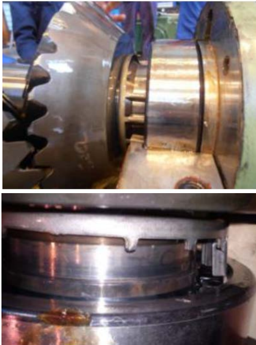
Figure 2. Damaged bearing on input shaft.
