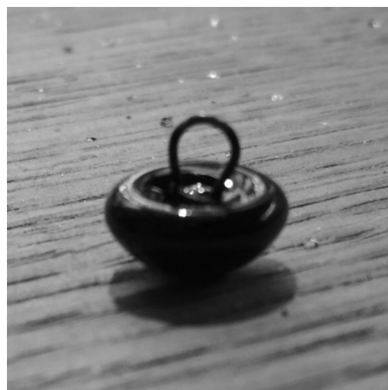
Figure 1: Produced black glass eye with wire loop
