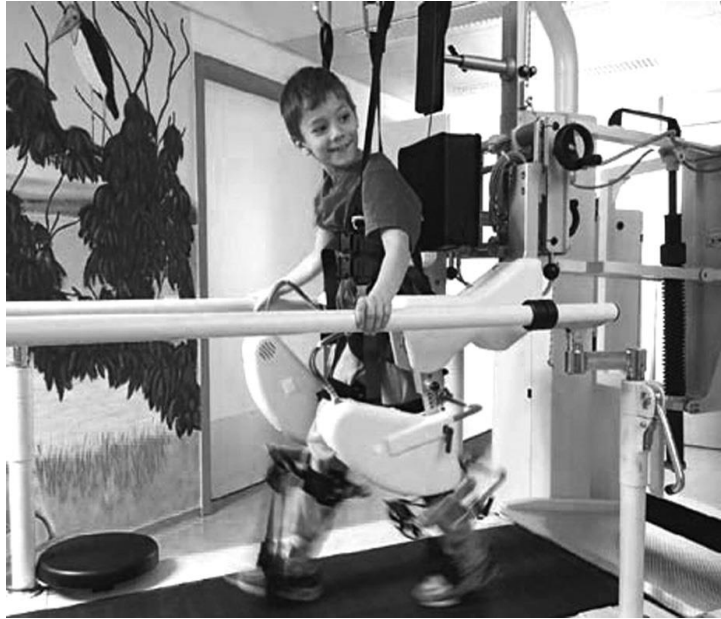
Figure 1: Robot Lokomat for strengthening the lower extremities
