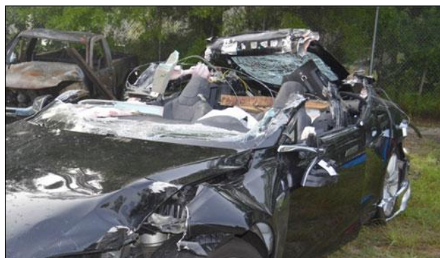
Figure 3: The unfortunate Tesla S - Passenger car damage from impact with semitrailer. (Source: Florida Highway Patrol.)
