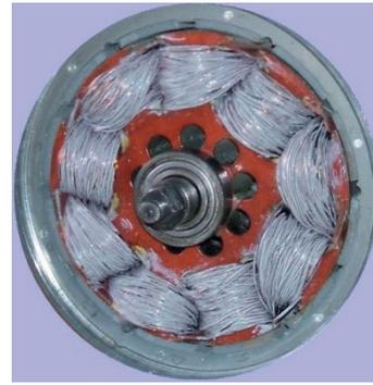
Figure 9 Photograph of prototype SMPM without bearing plate [8]
