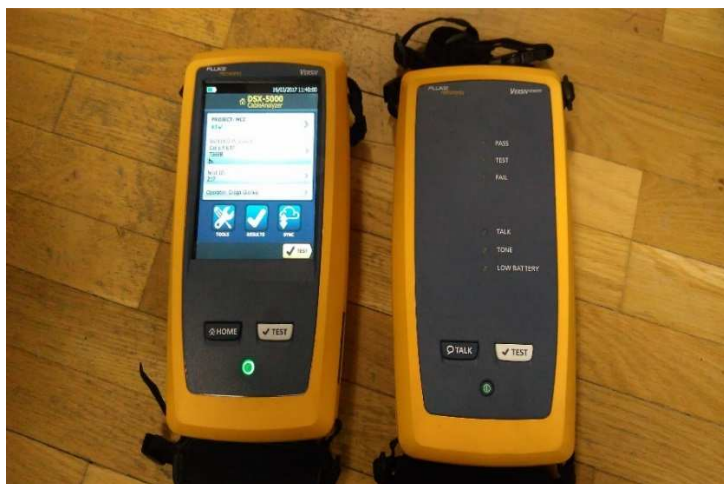
Picture 1. Instrument for measuring the telecommunication lines - Fluke 5000 Versio (author's source)
