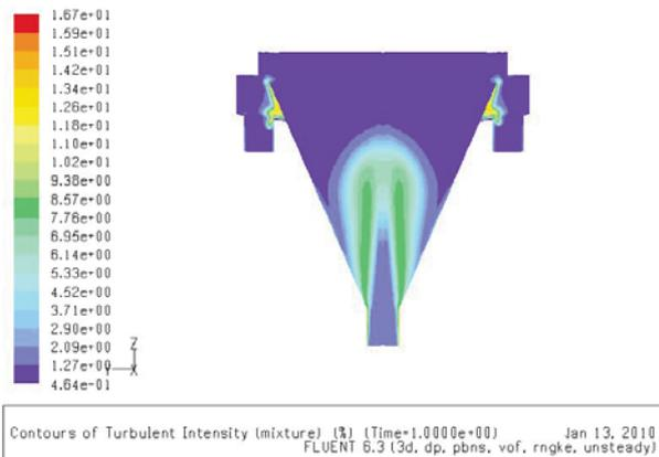
Fig. 10 Turbulent intensity in the time of 1 s
