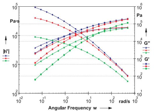
PP before exposure, PP 500 exposed in n-hexane (0 - 300 μm), PP 500 exposed in n-hexane (300 - 600 μm)
