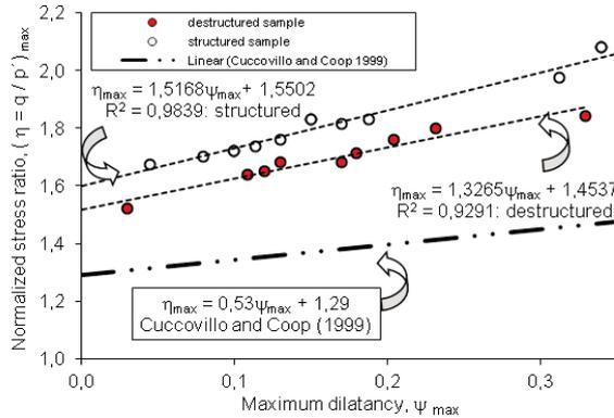
Fig. 7 Stress-dilatancy data for destructured dense sample, structured sample of residual granitic residual soil and the same relationship obtained from Cuccovillo and Coop (1999)
