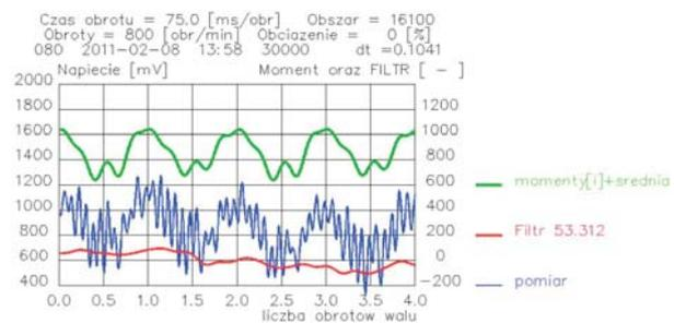
Fig. 8. The course of torque measured with the torque sensor - the thinnest blue line, torque obtained after excluding harmonic components which are the multiplicity of the 720 degrees working cycle - the thickest green line, the sum of harmonic components excluded from the measured signal - red average thickness line; the courses obtained from measurement point nr 16100
