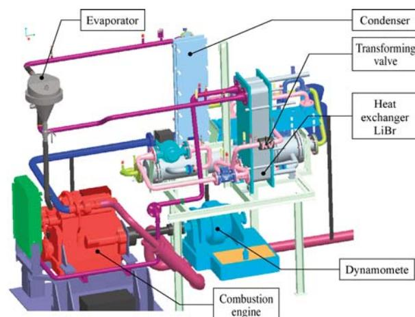
Fig. 1 Virtual model of the non-conventional energetic unit [2]
