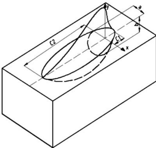
Fig. 2 Goldak double ellipsoidal heat source model [3]
