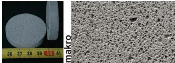
Fig. 1 Porous concrete PB specimens ready for measuring
