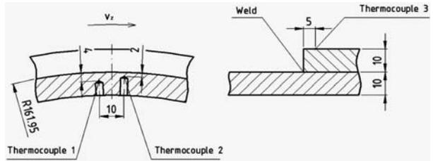
Fig. 6 Location of thermocouples
