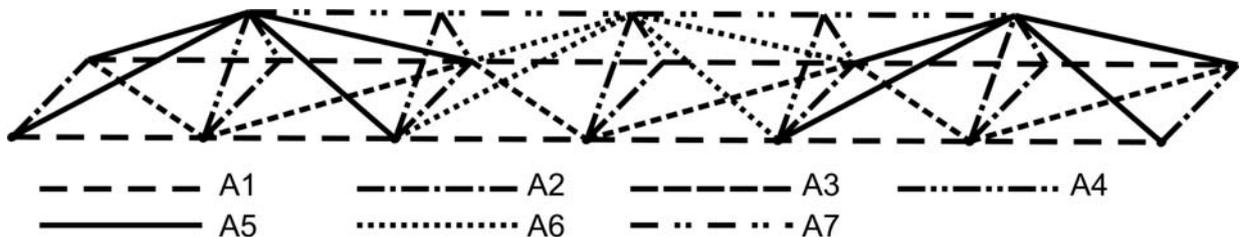
Fig. 6 Truss structure split into 7 cross-sectional groups
