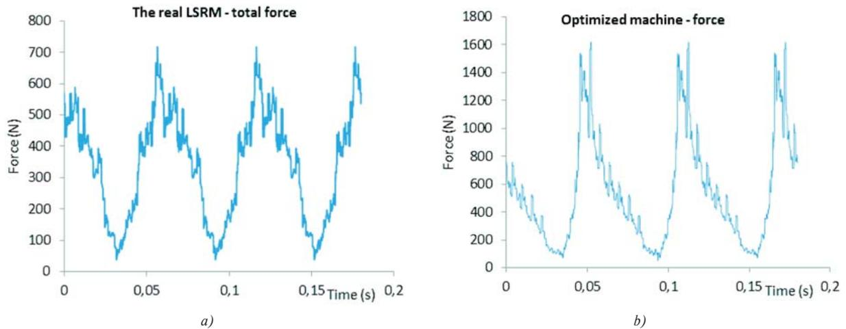
Fig. 12 The LSRM total electromagnetic force waveforms, a) real, b) optimized
