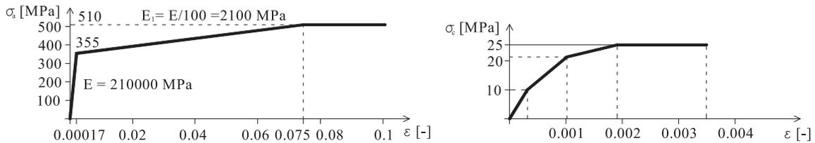
Fig. 2 Stress-strain curves of the steel and the concrete used in the FEM model
