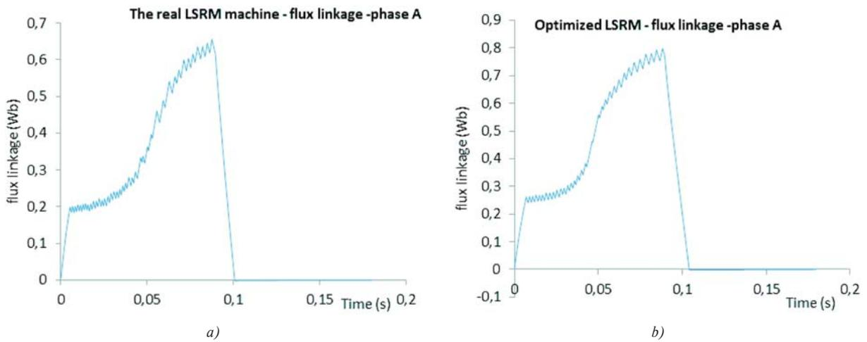
Fig. 11 The LSRM flux linkage waveforms, a) real, b) optimized
