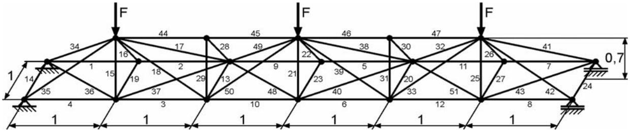
Fig. 5 Analyzed truss structure, dimensions in [m]
