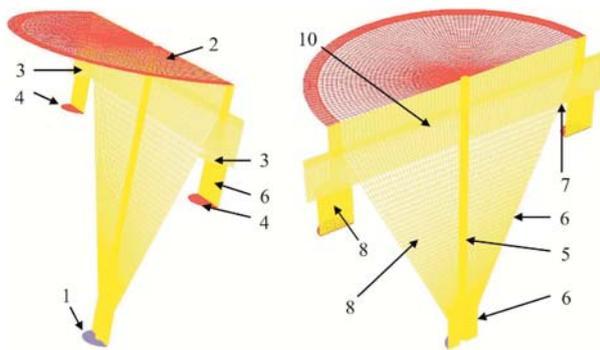
1-velocity inlet I, 2-pressure outlet I, 3-velocity inlet II, 4-pressure outlet II, 5-axis, 6-wall, 7-interface wall + velocity inlet II, 8-symetry
