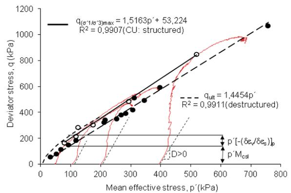
Fig. 9 Effective stress path for undrained tests on saturated granitic residual soil: failures envelopes for  $(\sigma'_1/\sigma'_3)_{max}$  and ultimate and intrinsic criterion of rupture
