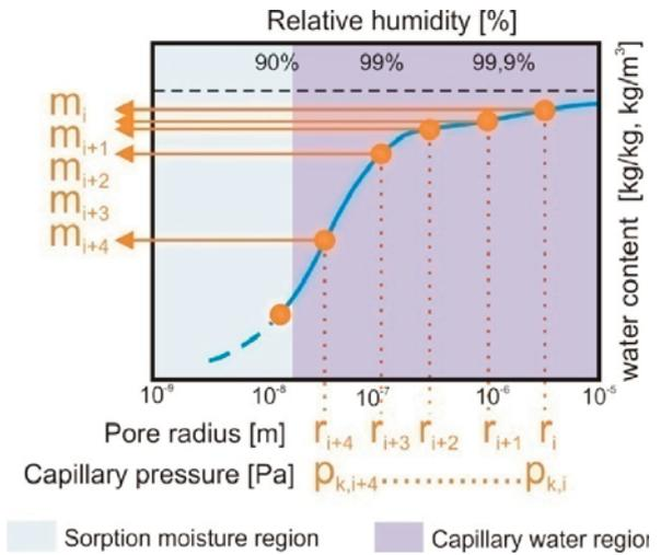
Fig. 5 Moisture storage function (suction curve) of a porous material
