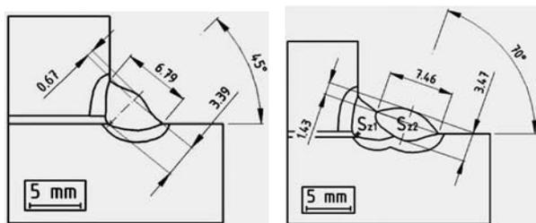
$S_{z1} = 17,2 \text{ mm}^2$  - weld area
