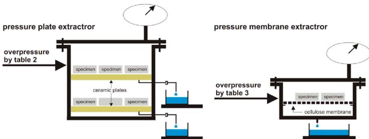
Fig. 7 Pressure plate (PPE) left and Pressure membrane (PME) extractor right
