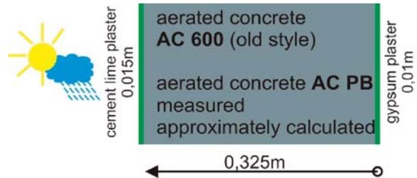
Fig. 3 Scheme of the analyzed building's envelope
