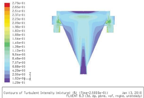
Fig. 11 Turbulent intensity in the time of 25 s
