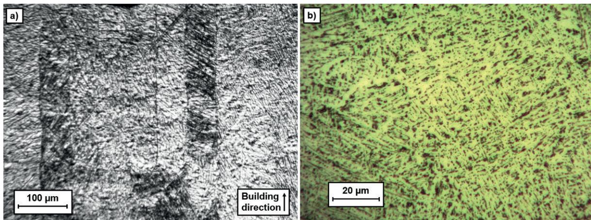
Figure 6 Microstructure of as-built Ti-6Al-4V AM sample
