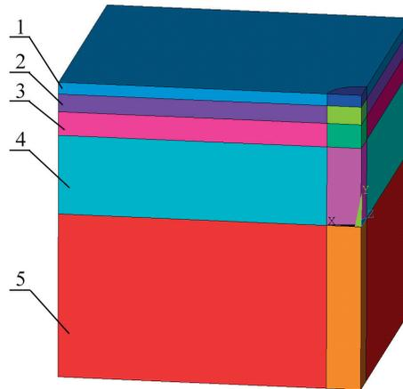
**Figure 2** Structural element of the pavement. The layers of the material correspond to the pavement layers shown in Figure 1
