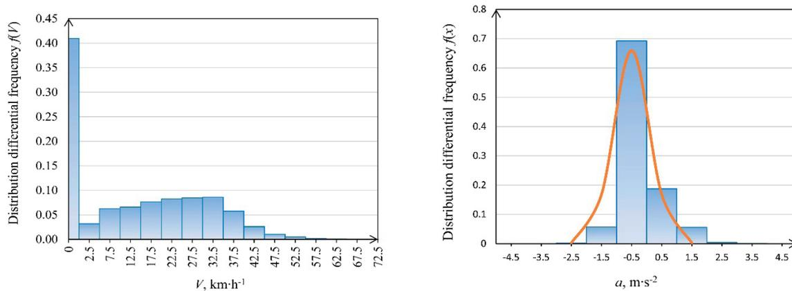
**Figure 5** Differential <sup>a</sup> distributions of bus speed and acceleration during the day: <sup>b</sup>  $a$  - speed,  $b$  - acceleration
