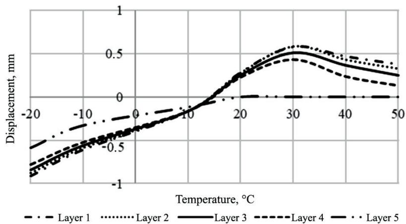
**Figure 6** Change in the maximum displacements in the layers of the road under the center of the contact area between the wheel and the road surface depending on the temperature of the upper layer  $T_i$ .
