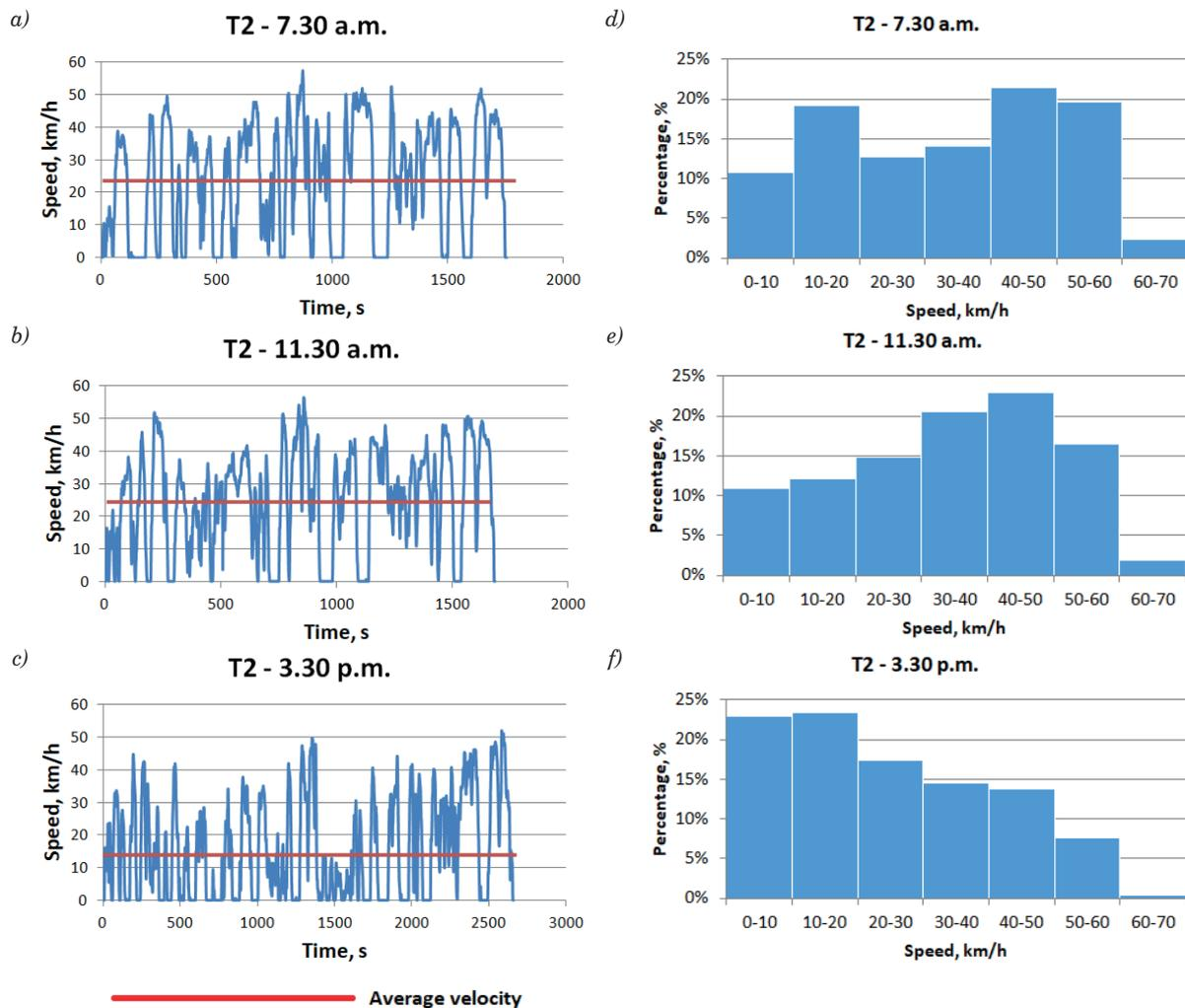
**Figure 5** Vehicle speed characteristics for route T2 in each of the analyzed hours: a - Vehicle speed profile at 7.30 a.m., b - Vehicle speed profile at 11.30 a.m., c - Vehicle speed profile at 3.30 p.m.; d - Vehicle speed distribution at 7.30 a.m., e - Vehicle speed distribution at 11.30 a.m., f - Vehicle speed distribution at 3.30 p.m.
