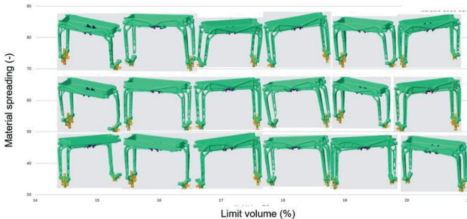
Figure 4 Effect of material spreading and limit volume parameters to the design
