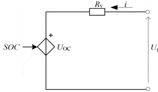
**Figure 1** Equivalent circuit of a battery cell
