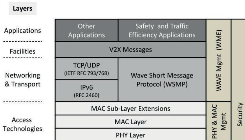
Figure 3 Communication model for WAVE protocol [2]
