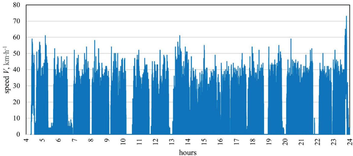
**Figure 4** Bus speed profile during the day
