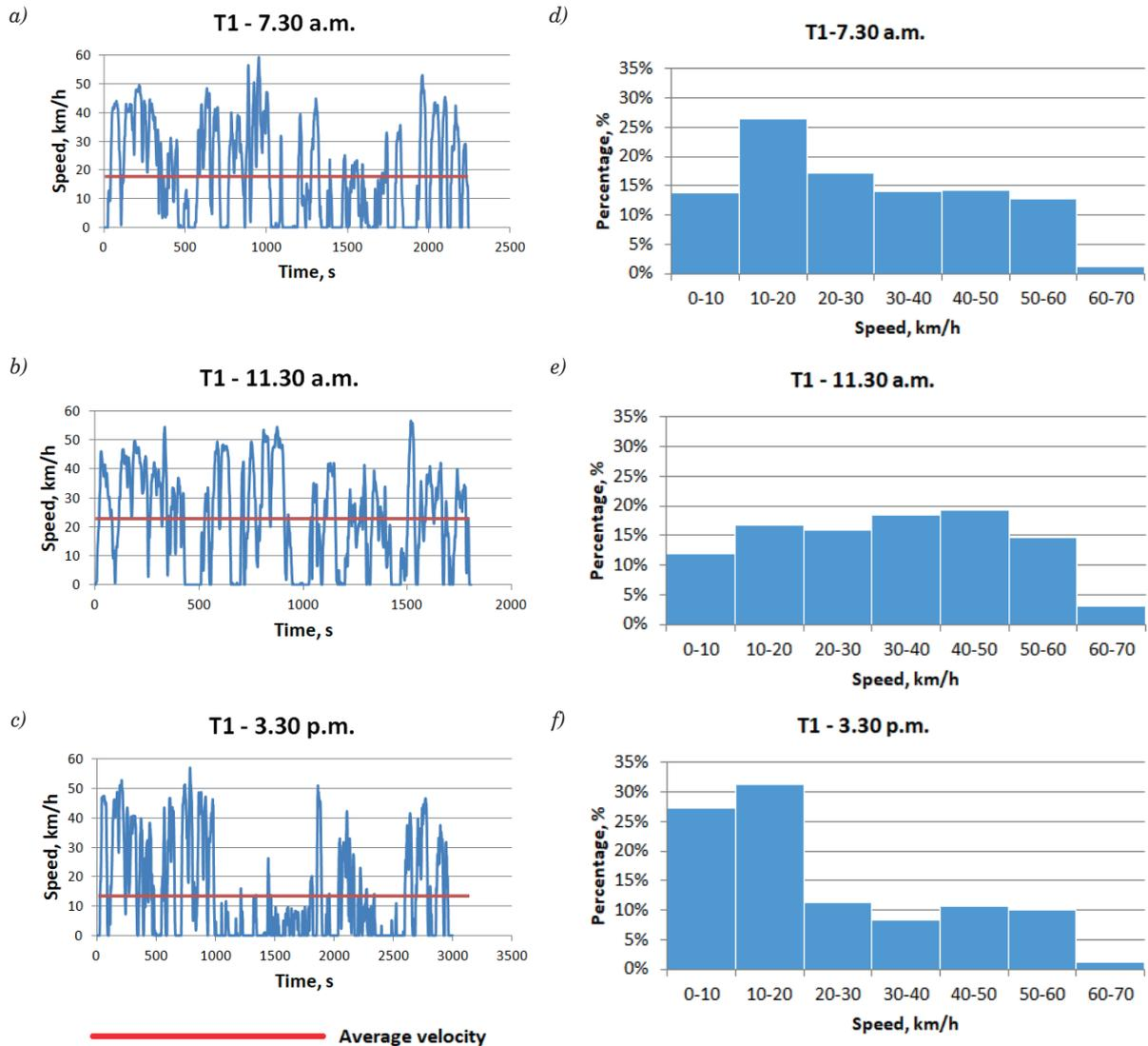
**Figure 4** Vehicle speed characteristics for route T1 in each of the analyzed hours: a - Vehicle speed profile at 7.30 a.m., b - Vehicle speed profile at 11.30 a.m., c - Vehicle speed profile at 3.30 p.m.; d - Vehicle speed distribution at 7.30 a.m., e - Vehicle speed distribution at 11.30 a.m., f - Vehicle speed distribution at 3.30 p.m.
