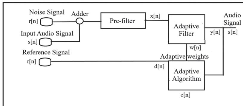
Figure 3 Proposed Active noise cancellation model with the pre-filter
