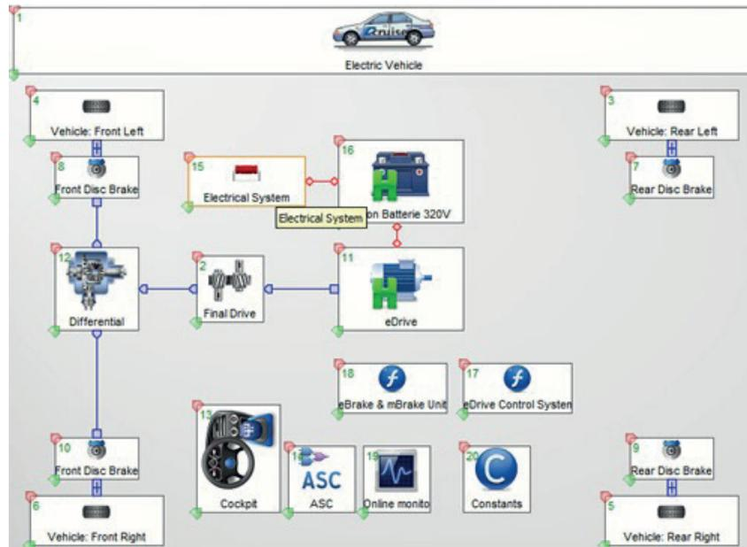
Figure 3 Electric vehicle model in AVL Cruise software
