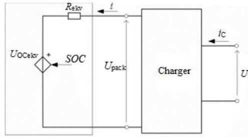
**Figure 2** Equivalent circuit of a battery
