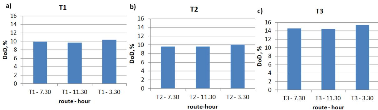
**Figure 8** Battery depth of discharge in the analyzed hours after completing routes a) T1, b) T2, c) T3
