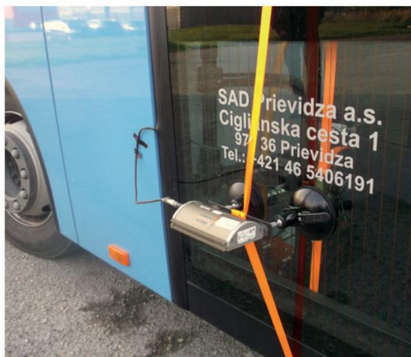
**Figure 1** Attachment of the microwave optical sensor
