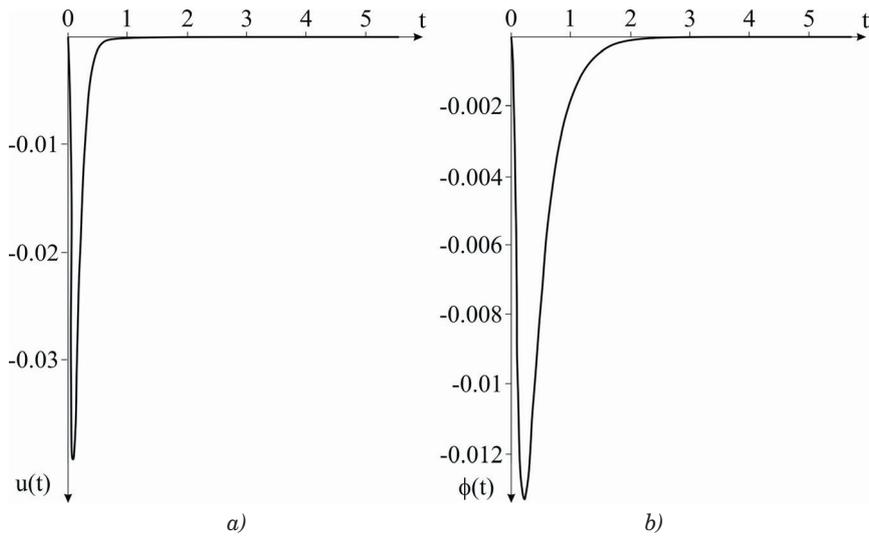
**Figure 2** Variation of the lateral velocity a) and folding angle b) during the transition process,  $v = 32 \text{ m/s}$
