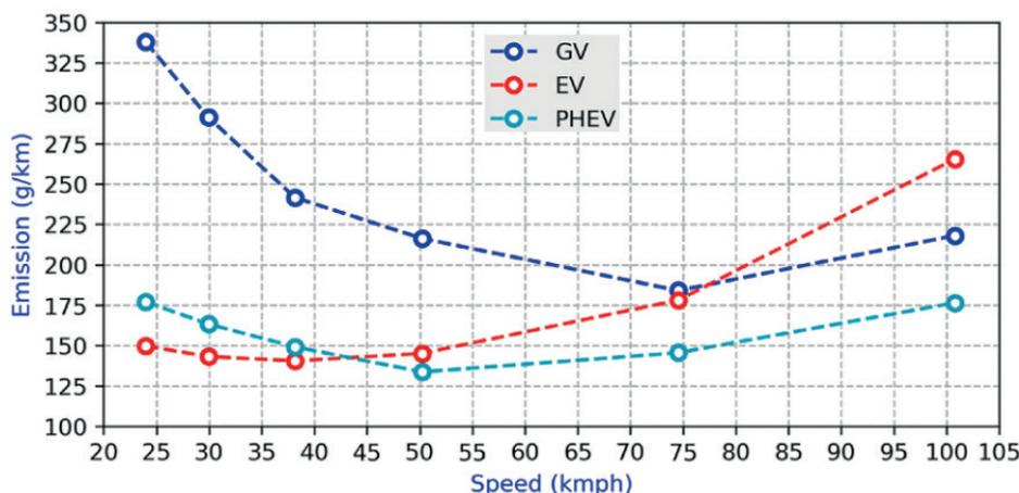
Figure 2 Emission versus speed plot of different vehicles for the Texas electricity generation mix [7]
