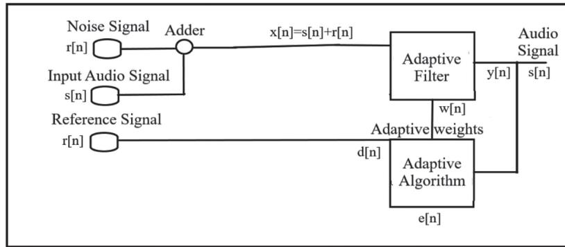
Figure 2 Active noise cancellation model without the pre-filter
