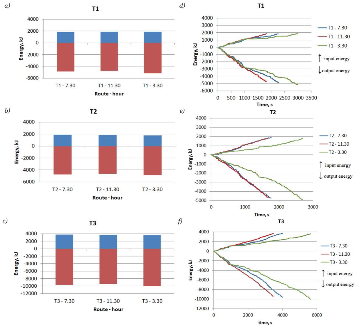
**Figure 7** Energy consumption of the vehicle during the drive: a, b, c - comparison of the input and output energy for the routes T1, T2 and T3, respectively in the tested hours, e, f, g - the curve of the input and output energy consumption for routes T1, T2 and T3, respectively
