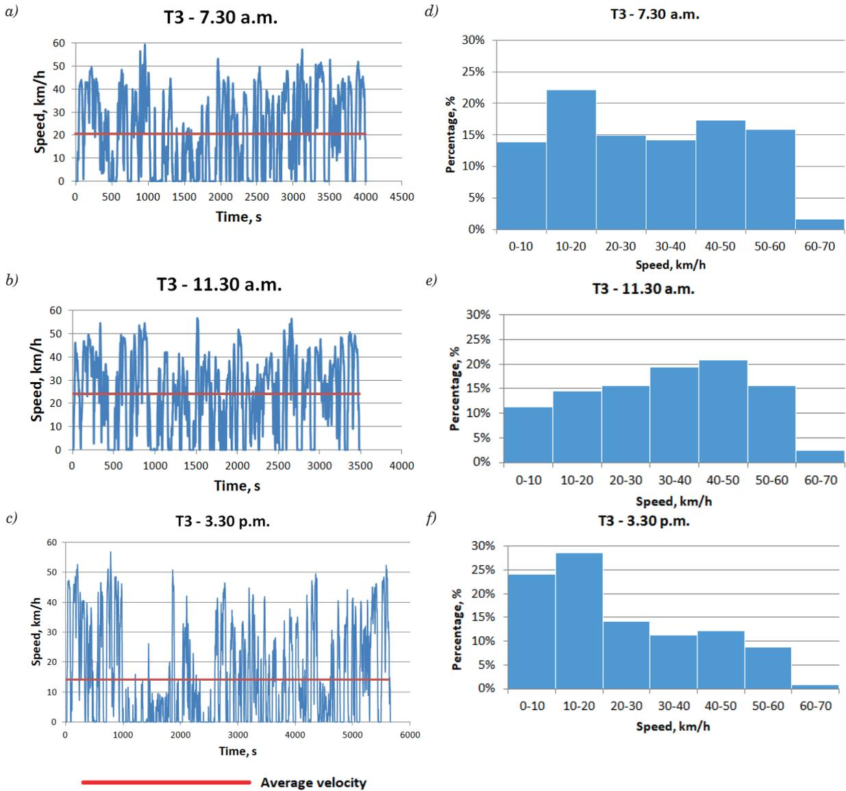
**Figure 6** Vehicle speed characteristics for route T3 in each hour analyzed: a - Vehicle speed profile at 7.30 a.m., b - Vehicle speed profile at 11.30 a.m., c - Vehicle speed profile at 3.30 p.m.; d - Vehicle speed distribution at 7.30 a.m., e - Vehicle speed distribution at 11.30 a.m., f - Vehicle speed distribution at 3.30 p.m.
