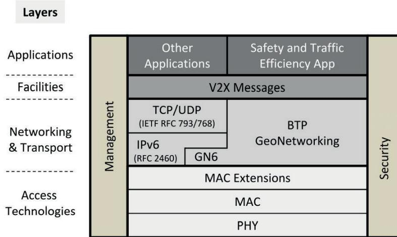
Figure 5 Communication model for the ETSI ITS protocol [2]
