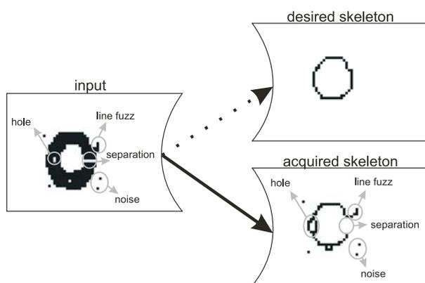
Fig. 2 Desired and acquired skeleton of input image
