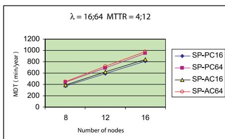
Fig. 13 MDT for Span Protection for MTTR=4; 12 h
