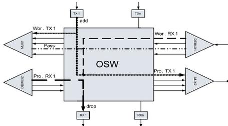
Fig. 6 Node structures with an active optical switch
