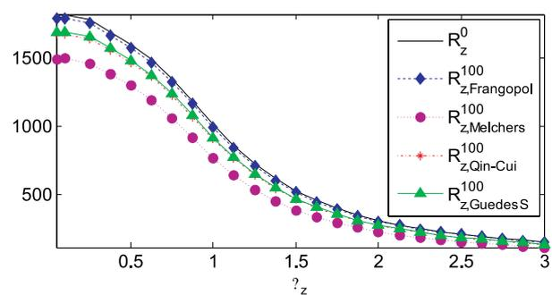
Fig. 2 The buckling resistances  $R_y$  and  $R_z$  in dependence on non-dimensional slenderness  $\bar{\lambda}$  for cross-section no. 2 (in zero time and after 100 years)
