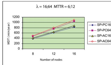
Fig. 14 MDT for Span Protection for MTTR=6; 12 h
