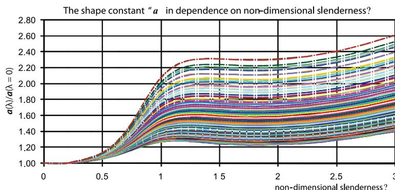
Fig. 4 The shape constant  $a$  in dependence on non-dimensional slenderness  $\bar{\lambda}$
