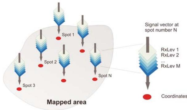
Fig. 1 Radio map for fingerprinting using RxLev
