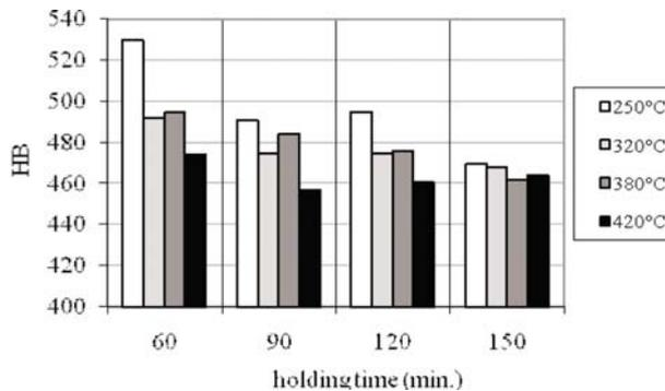
Fig. 5 Influence of temperature of isothermal transformation of austenite and holding time at this temperature on Brinell hardness
