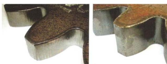
Fig. 3. Part of gearing produced by plasma arc at different thickness of gearing
