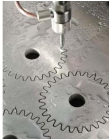
Fig. 5. Use of waterjet gear production
