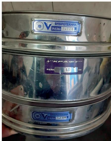
**Figure 7** Calibrated sieves from the Kraft Company
