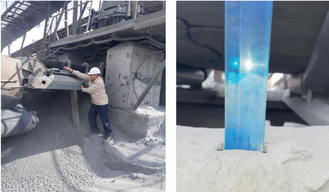
**Figure 5** Measuring technological dust in the CSC section
