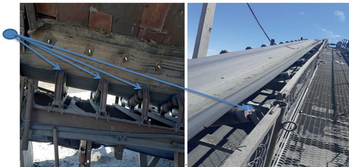
**Figure 8** Blue paint marks on the conveyor rollers
