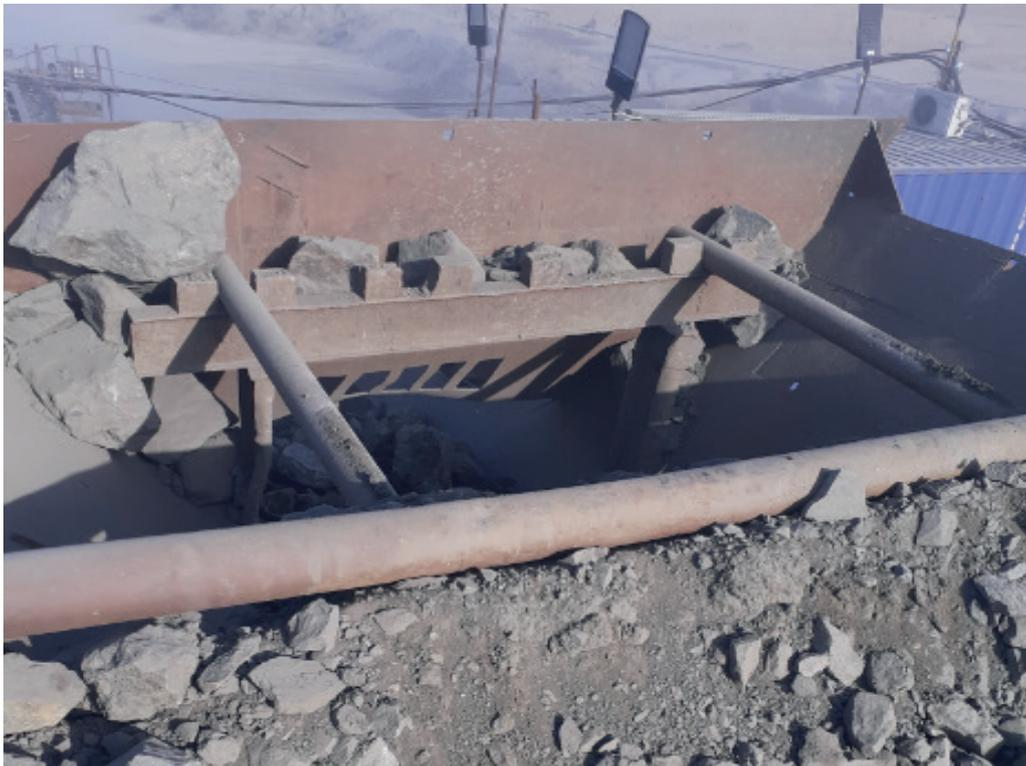
**Figure 3** Receiving hopper of the coarse lump crusher of the Maksut mine (position 6 of Figure 2) [9]
