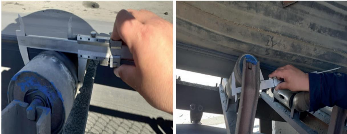
**Figure 9** Measuring the roller shell wear
