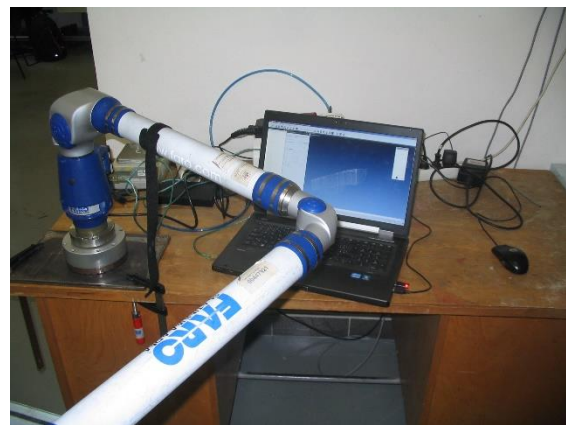
Obr. 2 Skener FARO Platinum Arm
