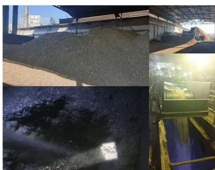
**Figure 3.** Dosing of solid recovered fuel into tank from landfill of Vojany black coal power plant. Source: Own processing by Vojany black coal power plant (2020).
