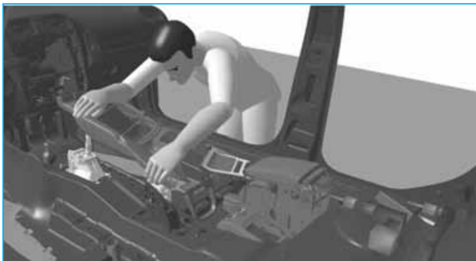
Obr. 1 Prepojenie modulov Delmia V5 DPM Assembly a V5 Human
