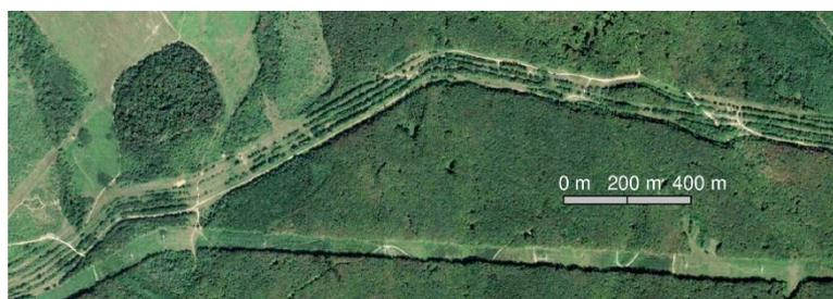
**Figure 2.** Part of parallel underground lines of the Eustream transport network recognizable on a satellite image.
