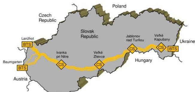
**Figure 1.** Scheme of the Eustream transport network on the territory of the Slovak Republic, where: CS—compressor station, BTS—border transfer station.
