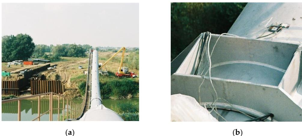
**Figure 5.** (a) View on the self-supporting pipeline in the direction of gas flow; (b) Detail of the applied strain gauges at the foundation footing.
