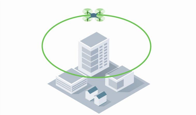
Figure 11. Circular flight plan
