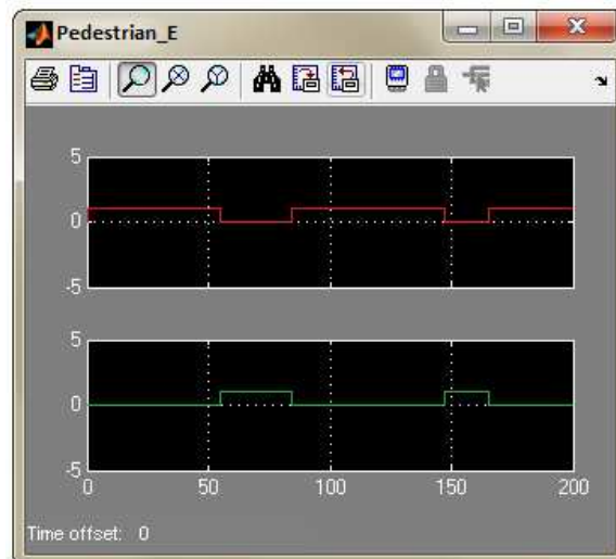
Figure 2: The form of the signals for crossing of the pedestrians
