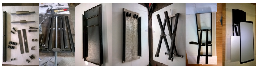
Figure 10. Production process of the leg lifter.
