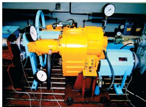
Fig. 2. Gearbox at the test stand
