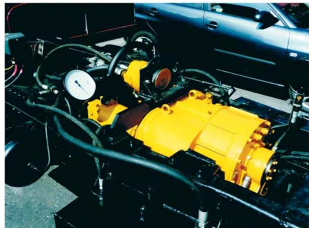
Fig. 4. The IVT 150 installed to the truck frame
