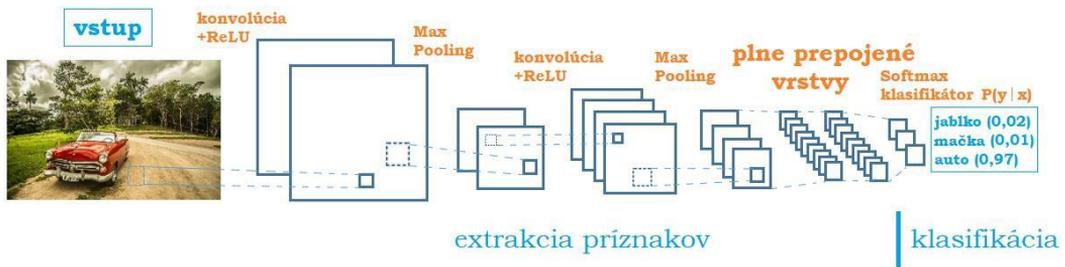
Fig.5. Simplified CNN operation procedure [8].
