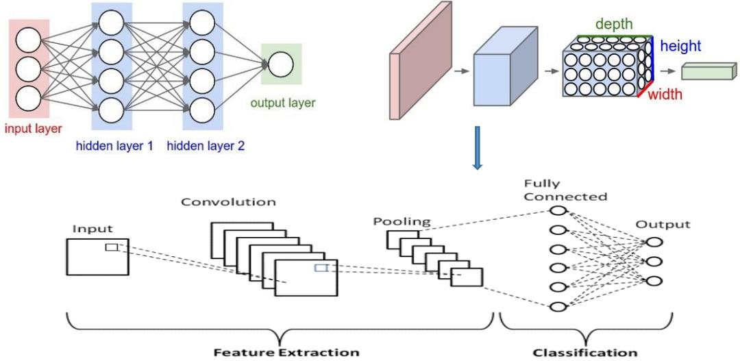
Fig.5. Conventional neural network (above left) and deep neural network structure.
