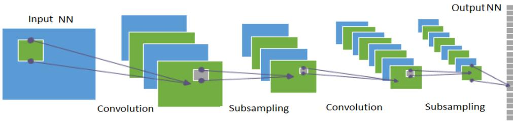
Fig.7. General convolution neural network architecture.
