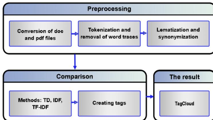
Fig.6. System architecture.
