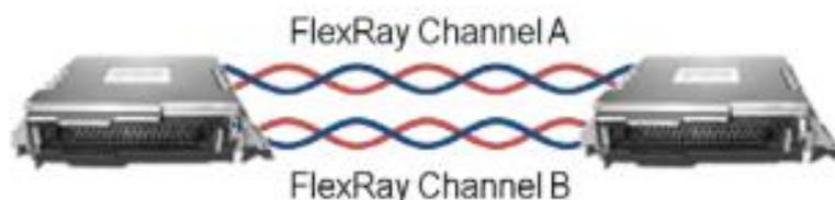
Fig. 1. FlexRay system basic communication structure.
