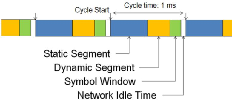
Fig.2. Communication cycle in FlexRay.
