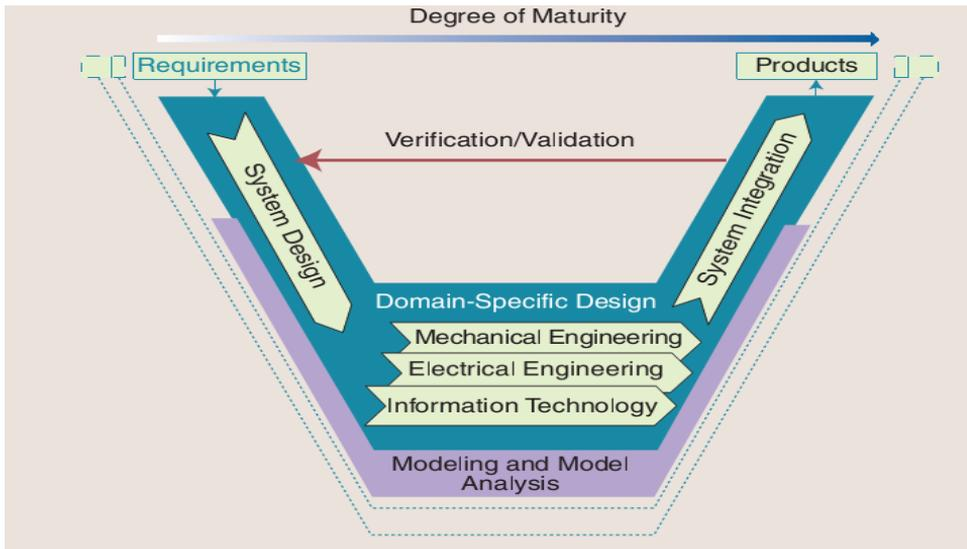
Fig.3. V-model scheme for development of mechatronic systems.
