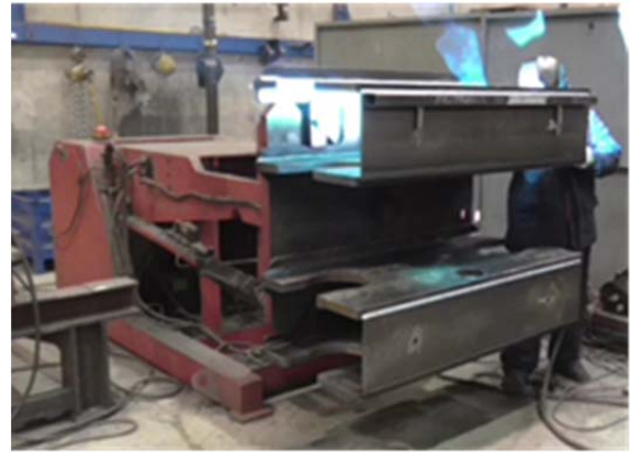
Figure 14. Original positioner for Fahrschemel welding
