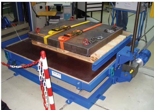
Fig. 3 Test for friction coefficients in laboratory in Germany
