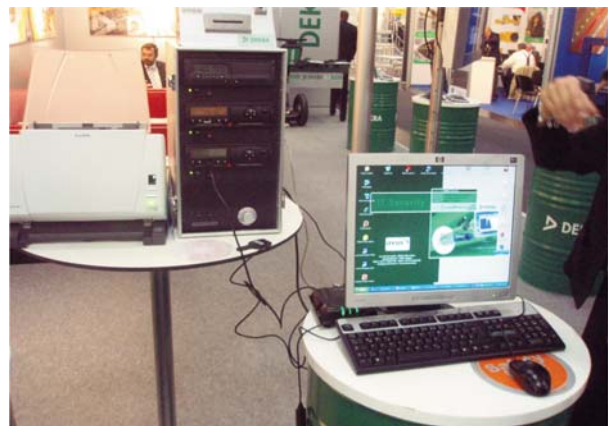
Fig. 4 Workplace for testing digital tachographs (example from DEKRA company)
