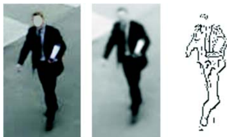
Fig. 6 The image shows the process of edges extraction. Blur is applied on original image, then Sobel edge detector is used. Detected edges serve as input for classification process.
