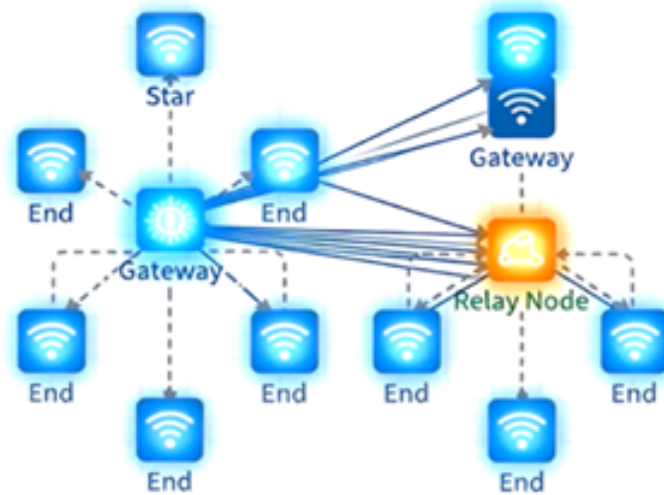
Figure 1. A typical cooperative relaying model used in LoRa networks
