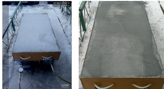
Figure 4 View of the bridge deck pavement experimental model before and after the research experiment with imitation of icing
