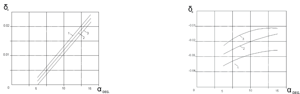
Figure 1 The dependence of certain parameters of the on-board slip coefficients of a 5VS-15M mechanical vehicle on the angle of rotation of the wheels
