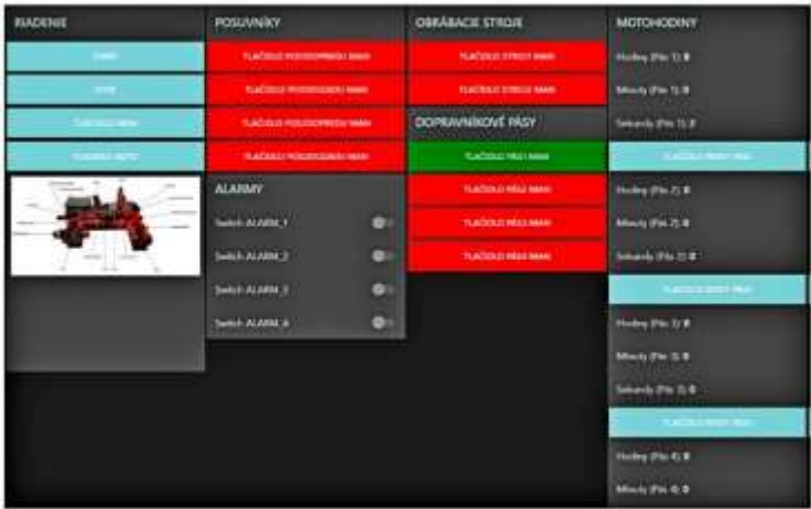
Fig.5. HMI in Node-Red environment during manual mode (MAN, AUTO buttons on left side). Four columns: Control, Sliders, Machines+Conveyors, Moto-hours.
