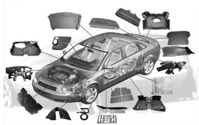
Figure 2. Textile material originally used in the automotive industry, which is recycled and used for production of STERED ® ( http://www.stered.sk , 2014)
