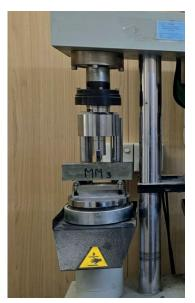
Figure 7 Flexural strength testing
