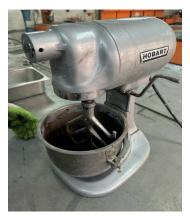
Figure 3 Mortar mixing process
