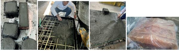
Figure 3 Casting, curing method for slab specimens
