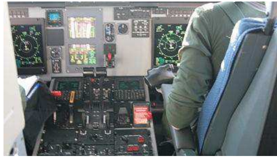
Figure 3 Pilot cabin of the CASA C-295 [7]
